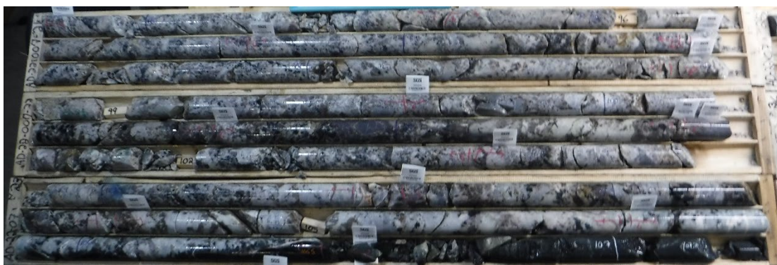
Photograph 1: Core recovery AD-22-007 – 94.7m to 107.1m Assays: 2.72% Li 2 O over 7.0m from 98.6m to 105.6m
