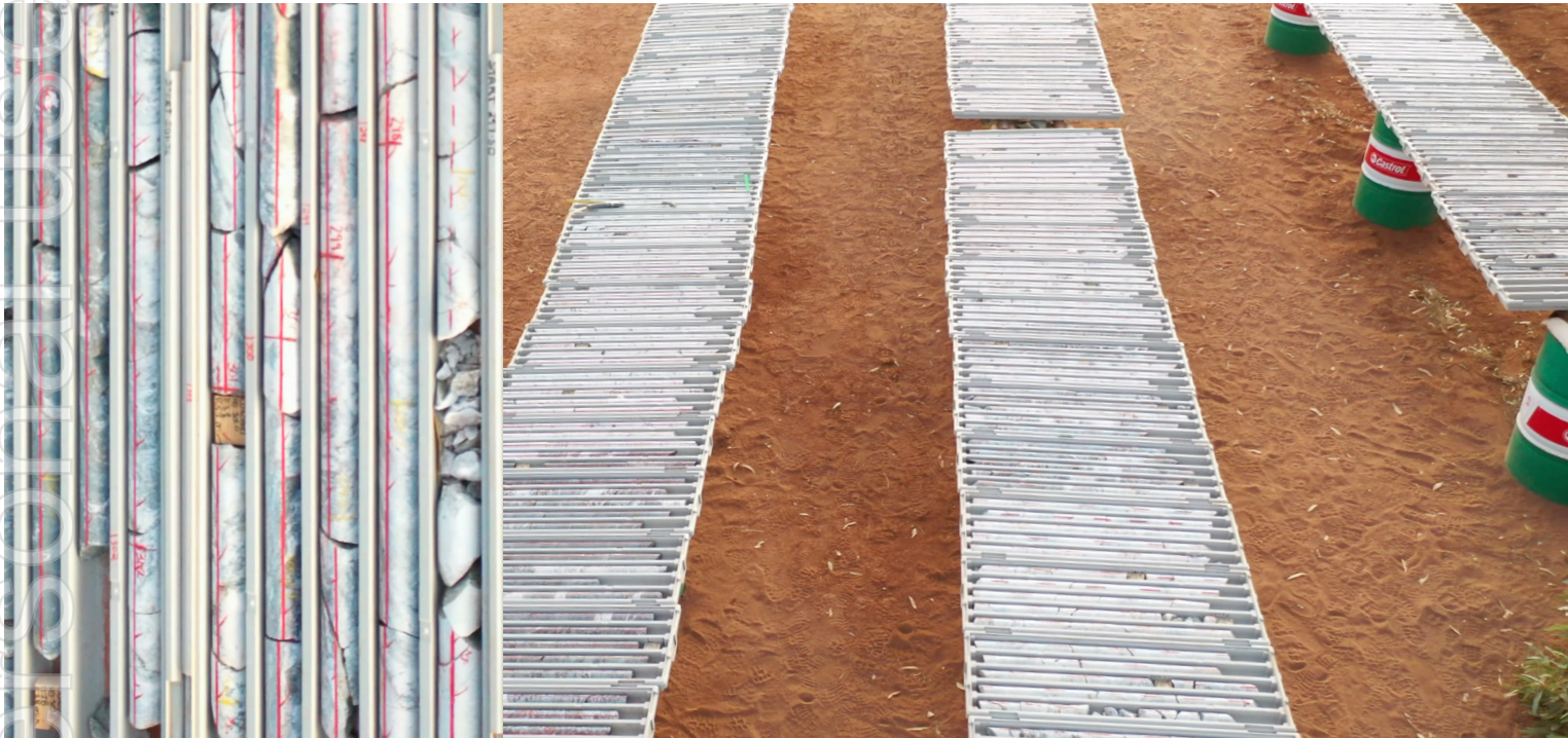
Top left: Orientated drill core from Cummins Range. Top right: Cummins Range drill core to be geologically logged.
