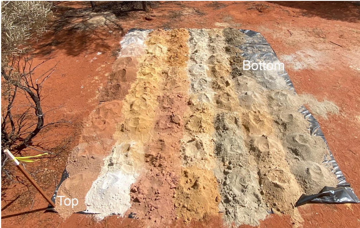
Figure 1. Reverse circulation samples from NSTRC071 showing colour variation due to oxidation in REE enriched regolith at North Stanmore
