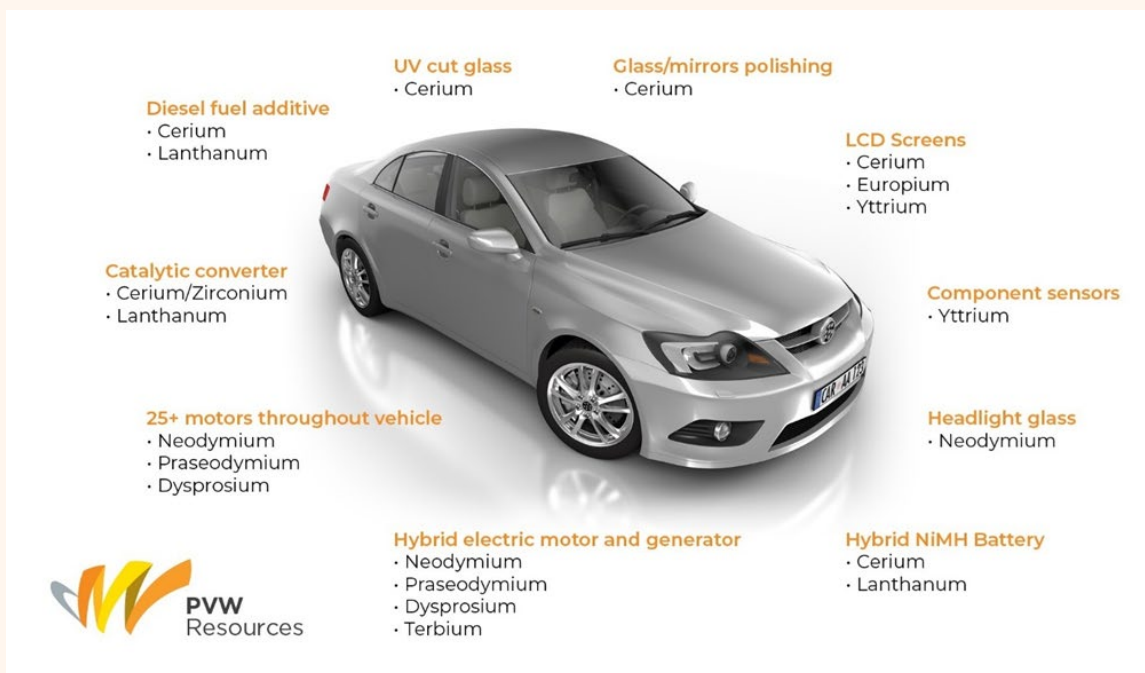
Figure 3: Rare earth elements used in electric vehicles
