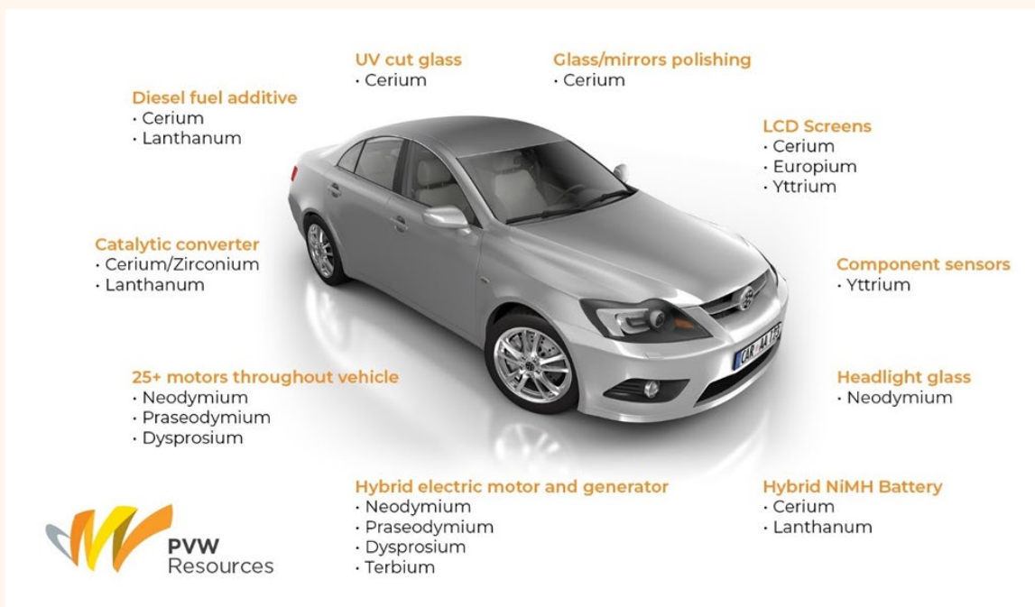
Figure 3: Rare earth elements used in electric vehicles
