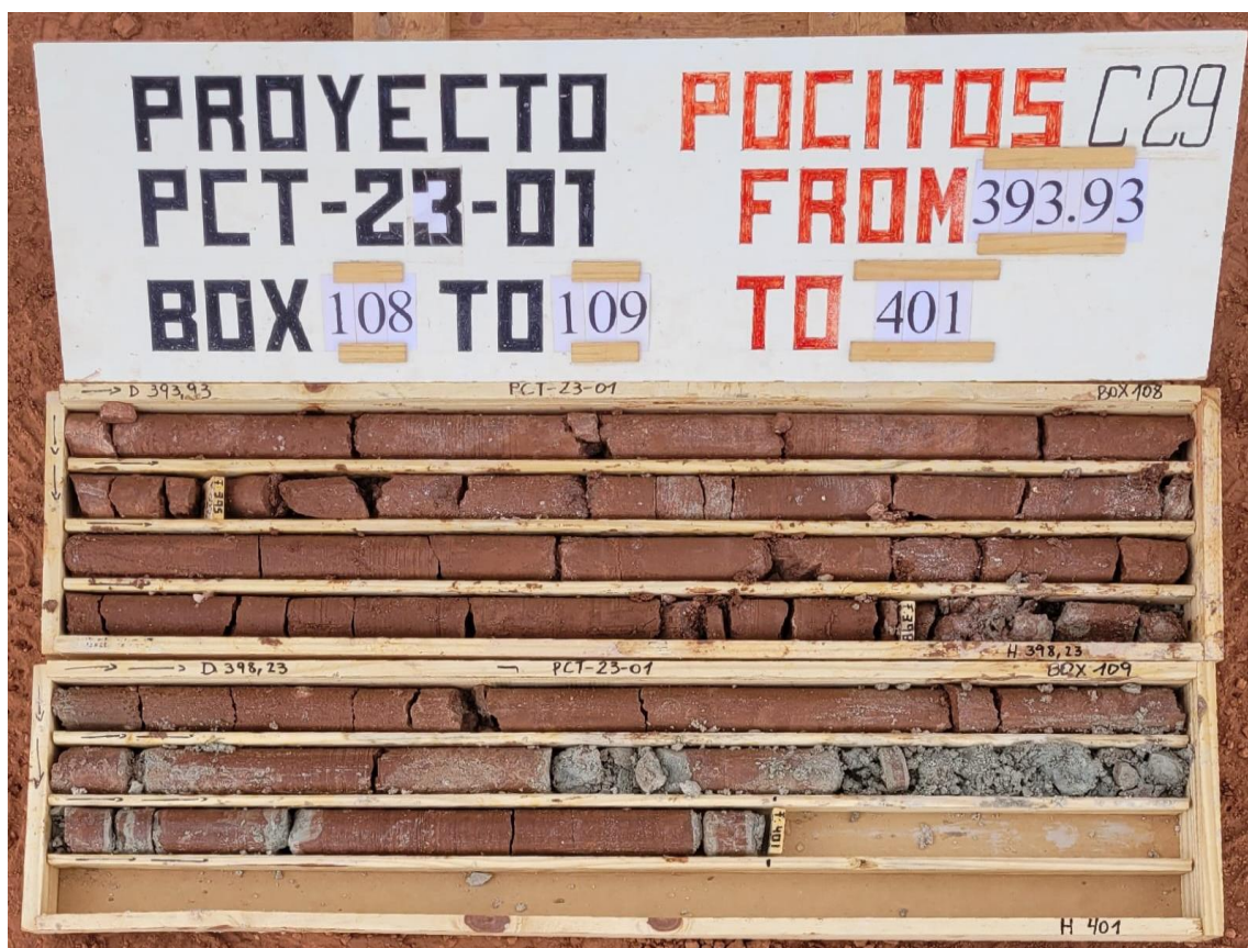
Figure 2: Core tray showing transition from clays to grey porous sand units
