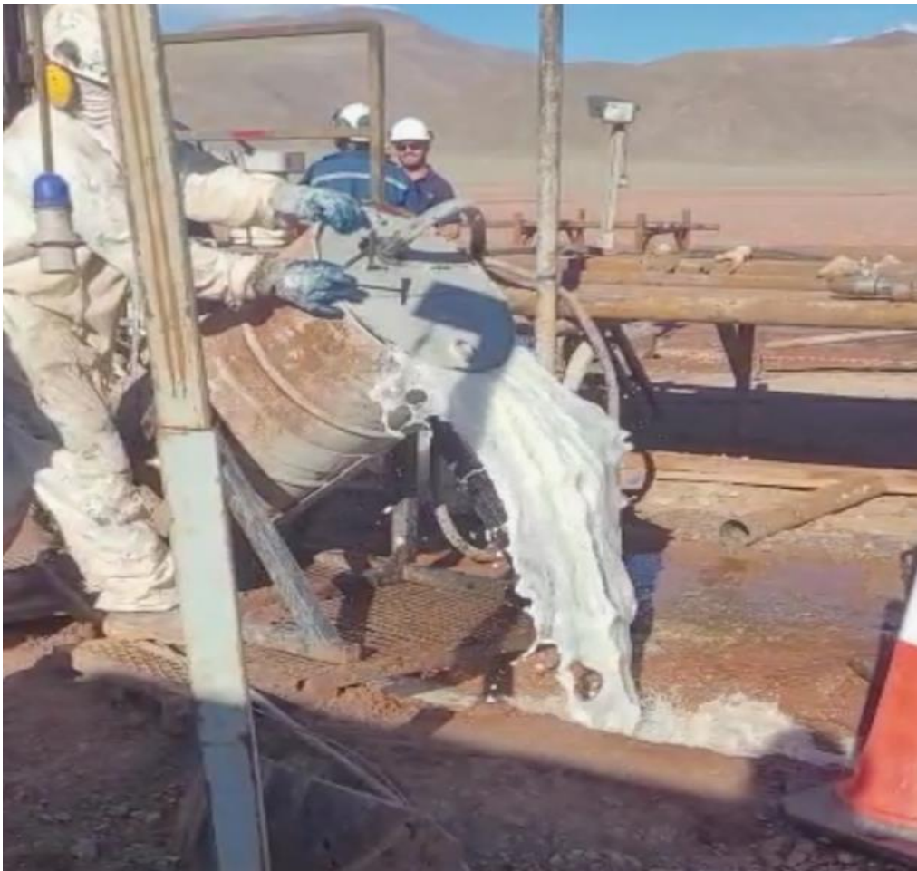
Figure 1: Brines being pumped into a 200l drum then emptied for the next measurement to be timed.
