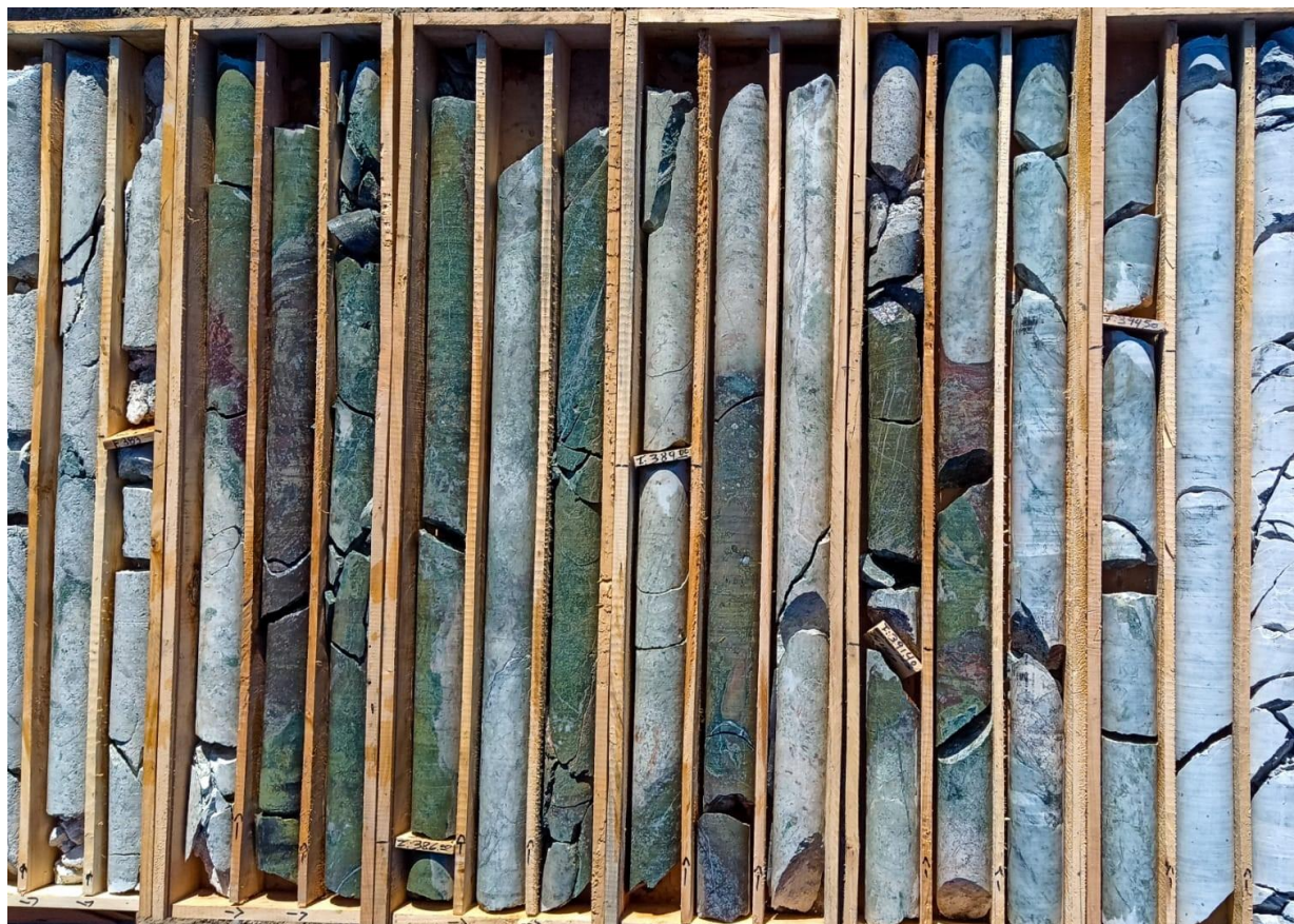
Image 2: GNDD-763 (Southern Verde Zone at depth) endoskarn alteration in intrusives (assays pending)
