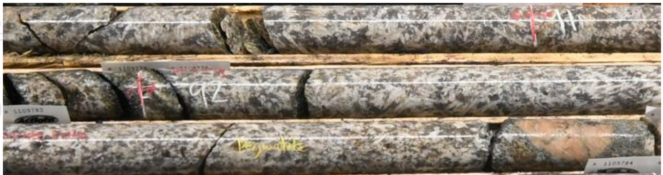
Figure 3: RL-22-0499: Whole NQ diamond core showing high density spodumene crystal laths, 7.2m @ 1.31% Li 2 O from 90.6m (incl. 3.2m @ 2.78% Li 2 O from 90.6m)
