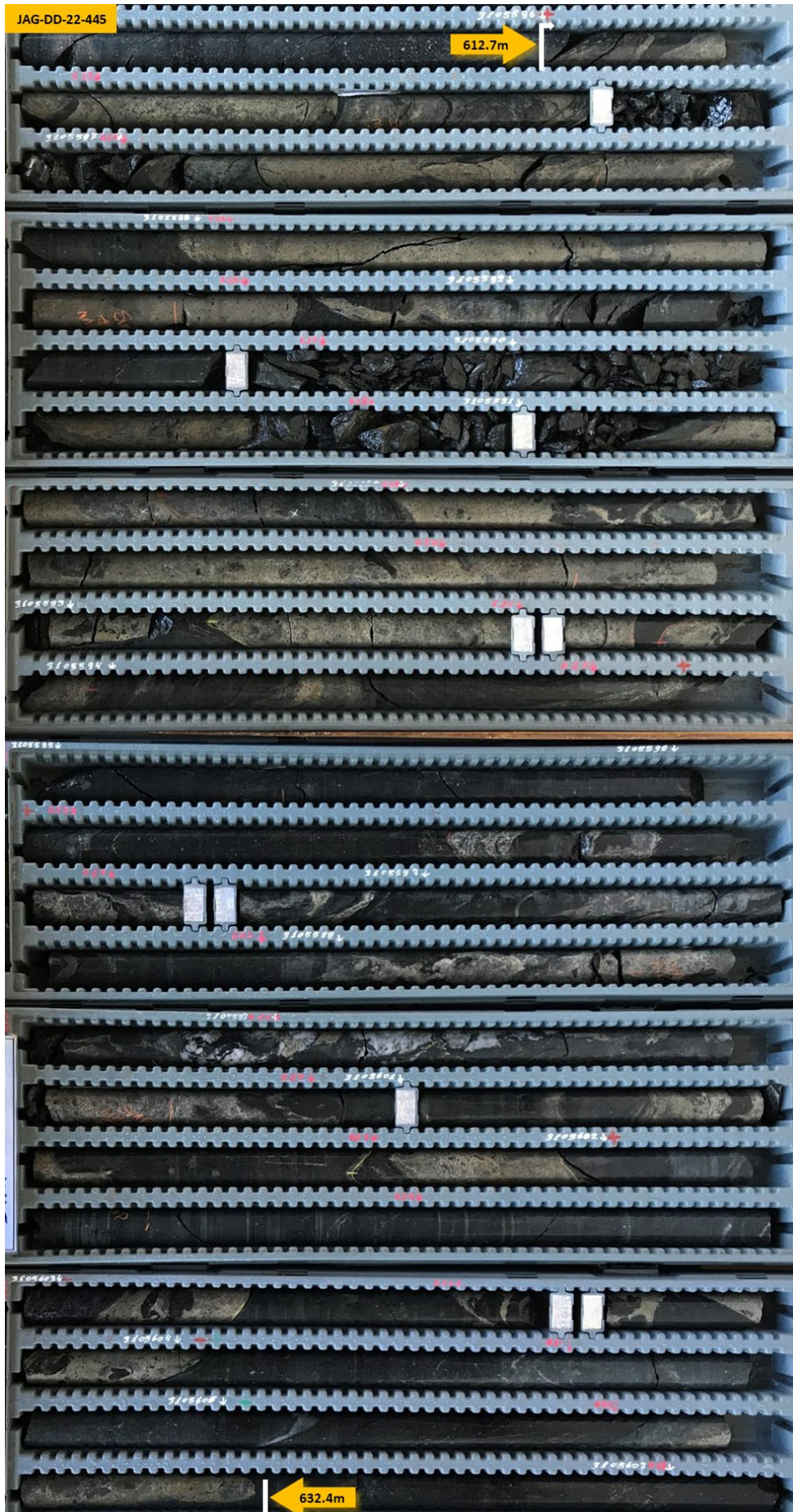
Figure 11 - The Jaguar South Deposit: Core photo from drill hole JAG-DD-22-445; 612.7m to 632.4m down-hole: Stringer, semi-massive and massive sulphides (dark metallic bronze) mineralisation with dacite host rock.
