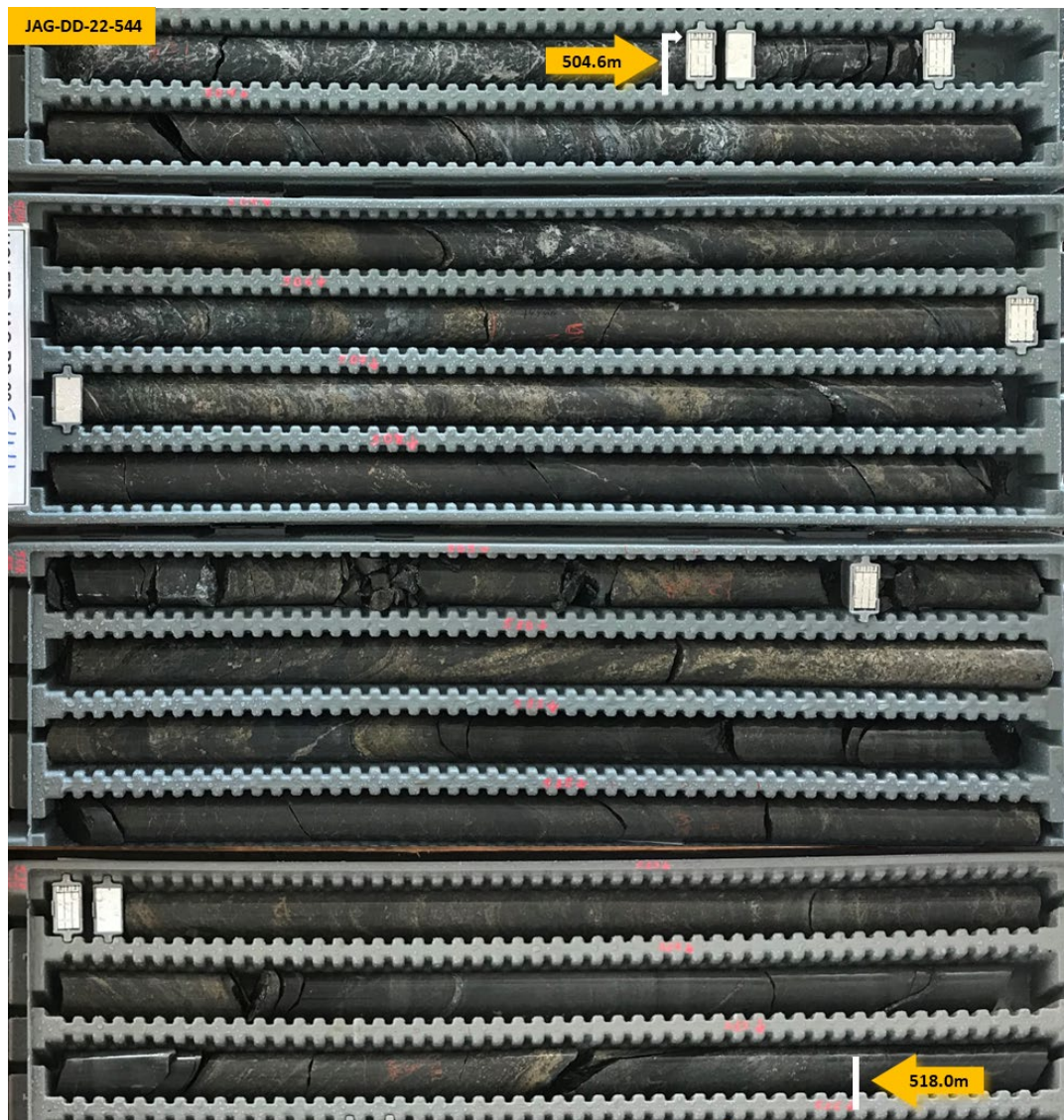
Figure 12 - The Onca Preta Deposit: Core photo from drill hole JAG-DD-22-544; 504.6m to 518.0m down-hole: Stringer, semi-massive and massive sulphides (dark metallic bronze) mineralisation associated with strong magnetite alteration (black).
