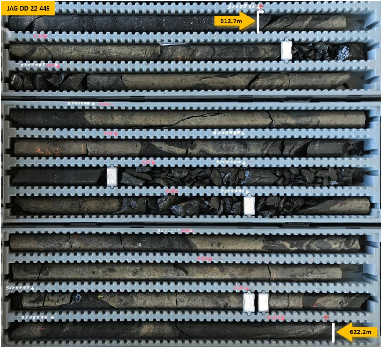
Figure 1 – The Jaguar South Deposit: Core photo from drill-hole JAG-DD-22-445; 612.7m to 622.2m down-hole: Stringer, semi-massive and massive sulphides (dark metallic bronze) mineralisation with dacite host rock.
