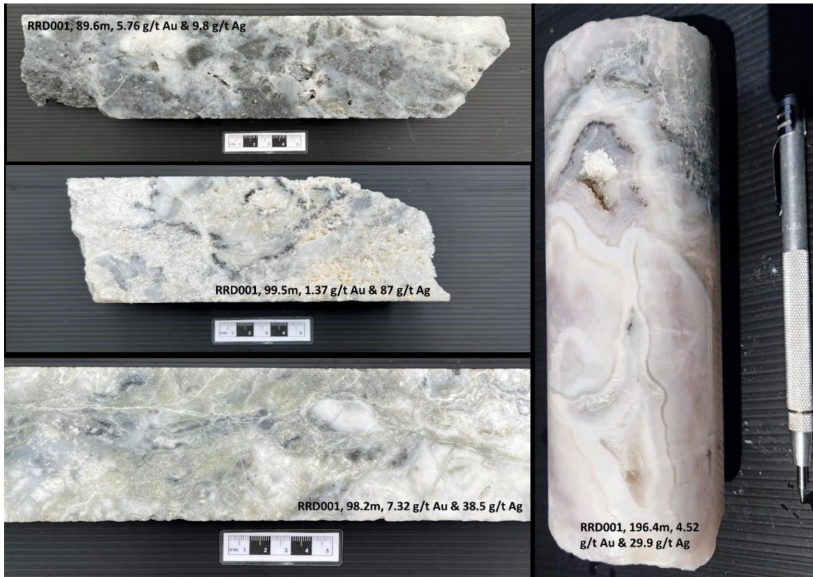
Figure 3: RRD001 drill core photos show examples of multiphase quartz veins as part of the Susi vein and presence of disseminated and thinly banded grey sulphide minerals. The vertical core specimen at right shows colloform banded quartz with pale amethyst. Assay results are indicated.
