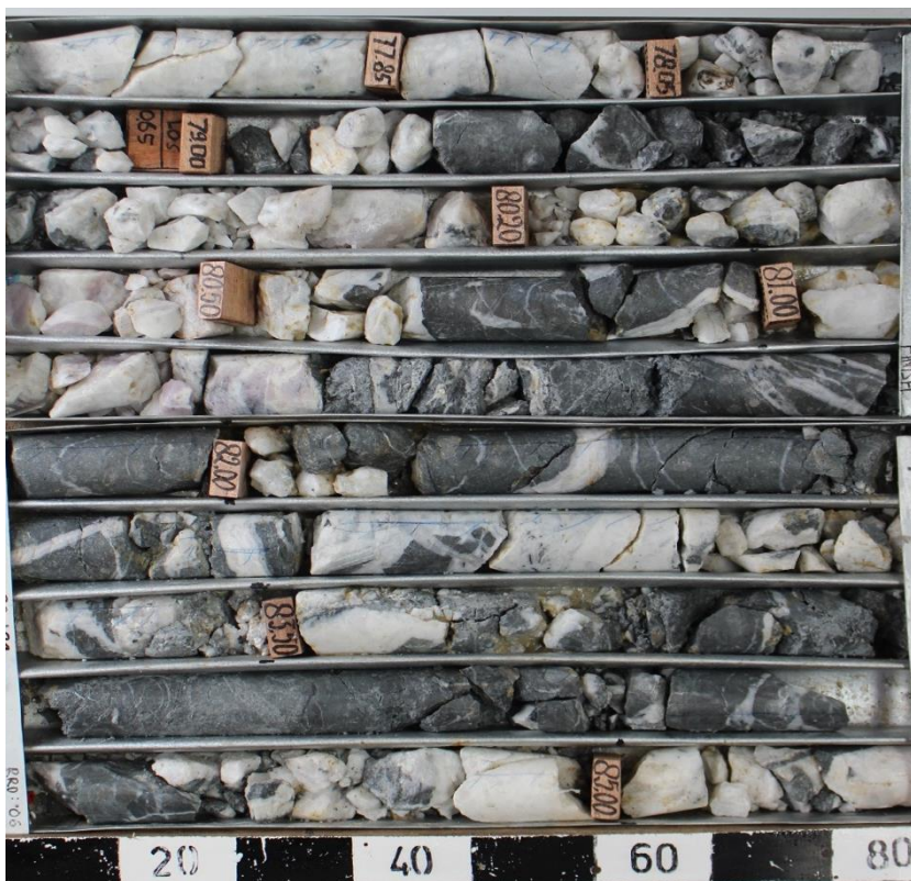
Figure 10: Section of drill core from RRD006 showing an approximate 5m section of the Susi vein zone. The section shows the occurrence of numerous finely banded crustiform quartz veins and bluish opaline veins adjacent to a zone of quartz breccia containing clasts of volcanic wallrock.
