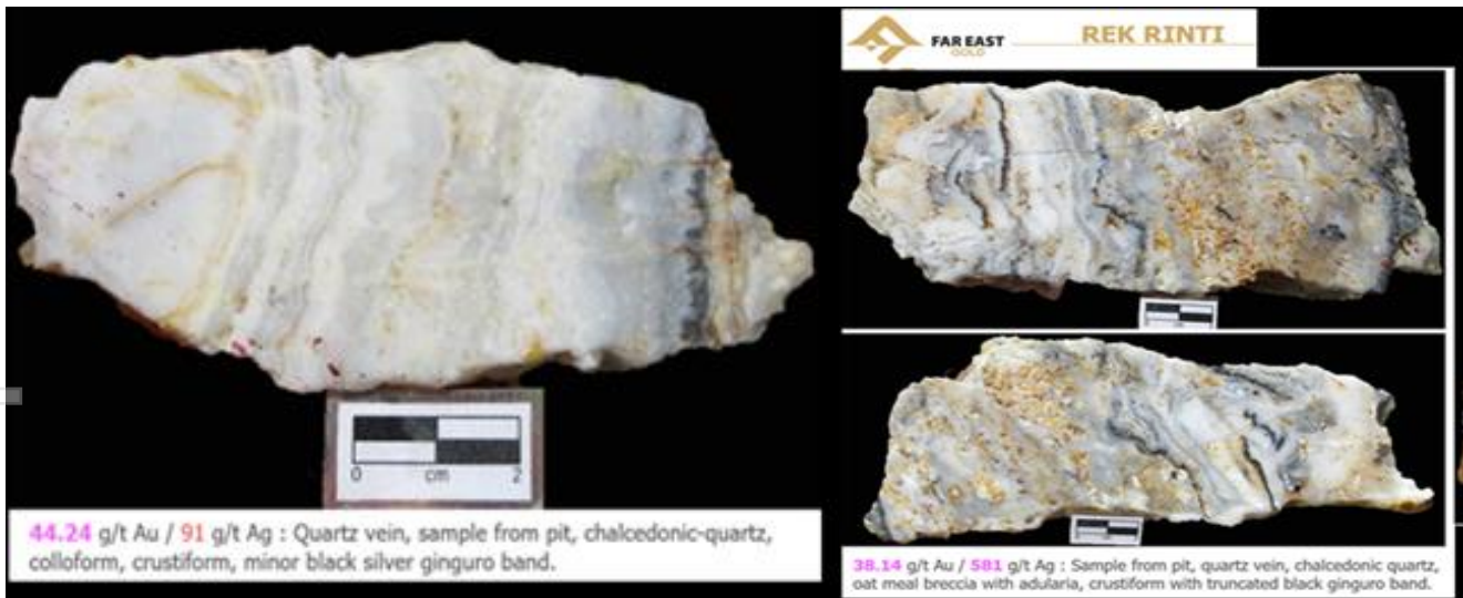
Figure 1: Examples of ginguro bands within samples of Rek Rinti quartz veins collected from surface and artisanal mining pits.
