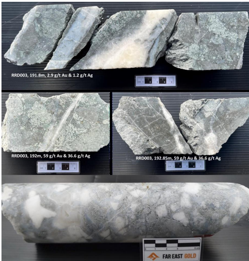
Figure 4: Core photos from deep (191.8m) high-grade gold intersection in RRD003. TOP: narrow crystalline quartz vein with possibly later opaline blue quartz veins at margin. MIDDLE: Narrow thinly banded crustiform quartz vein in chloritic lapilli tuff associated with high grade Au assay. BOTTOM: section of drill core from RRD003 (171m) showing presence of late, coarse white carbonate (calcite) infilling what were likely open cavities.
