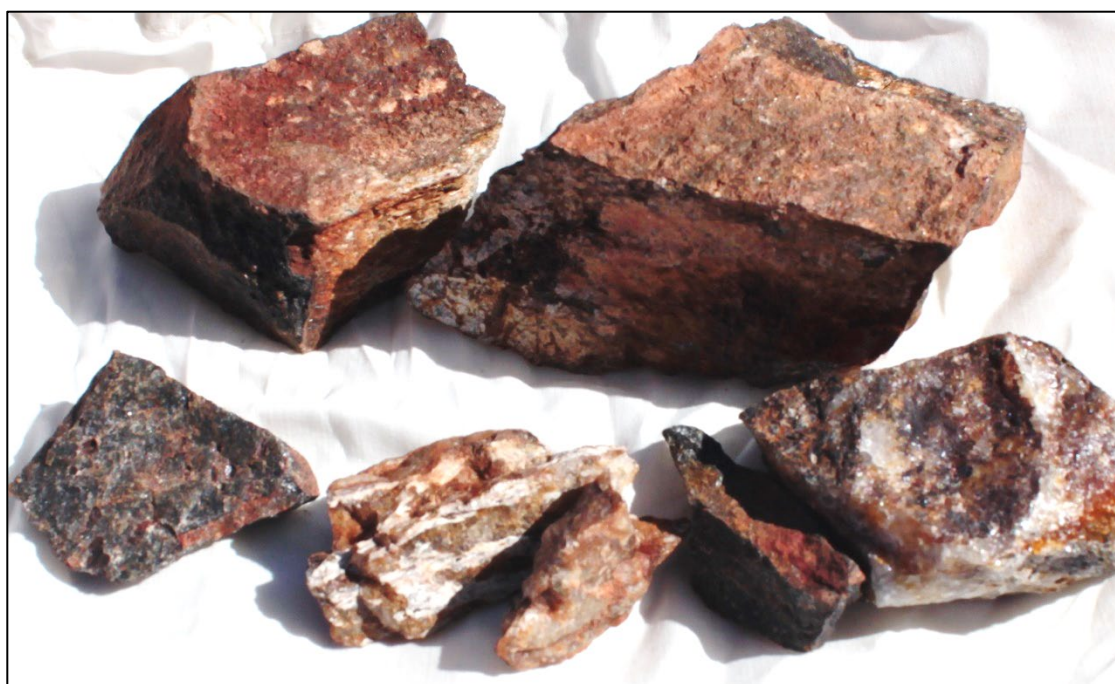
Figure 2: Photographs of mineralized rock samples containing combined quartz vein and silicified and iron oxide-rich vein wall rock material . Above: Sample 230103_3 grading 5.52g/t Au. Below: Sample 230103_10 grading 1.42g/t Au.
