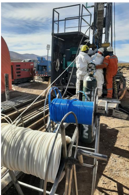
Figure 2: Packer sampling at SOZDD001
