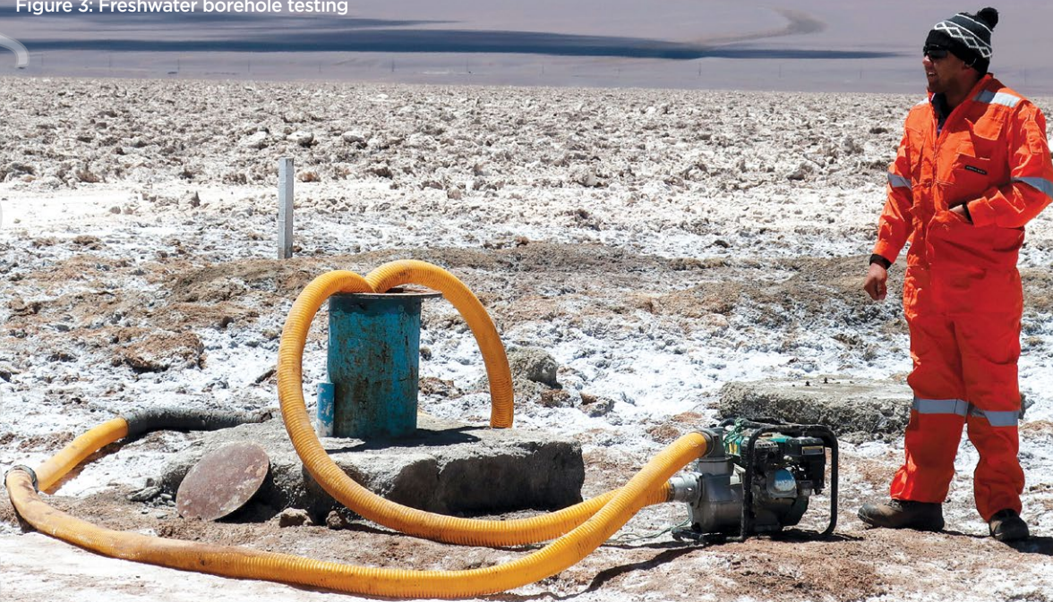
Figure 3: Freshwater borehole testing
