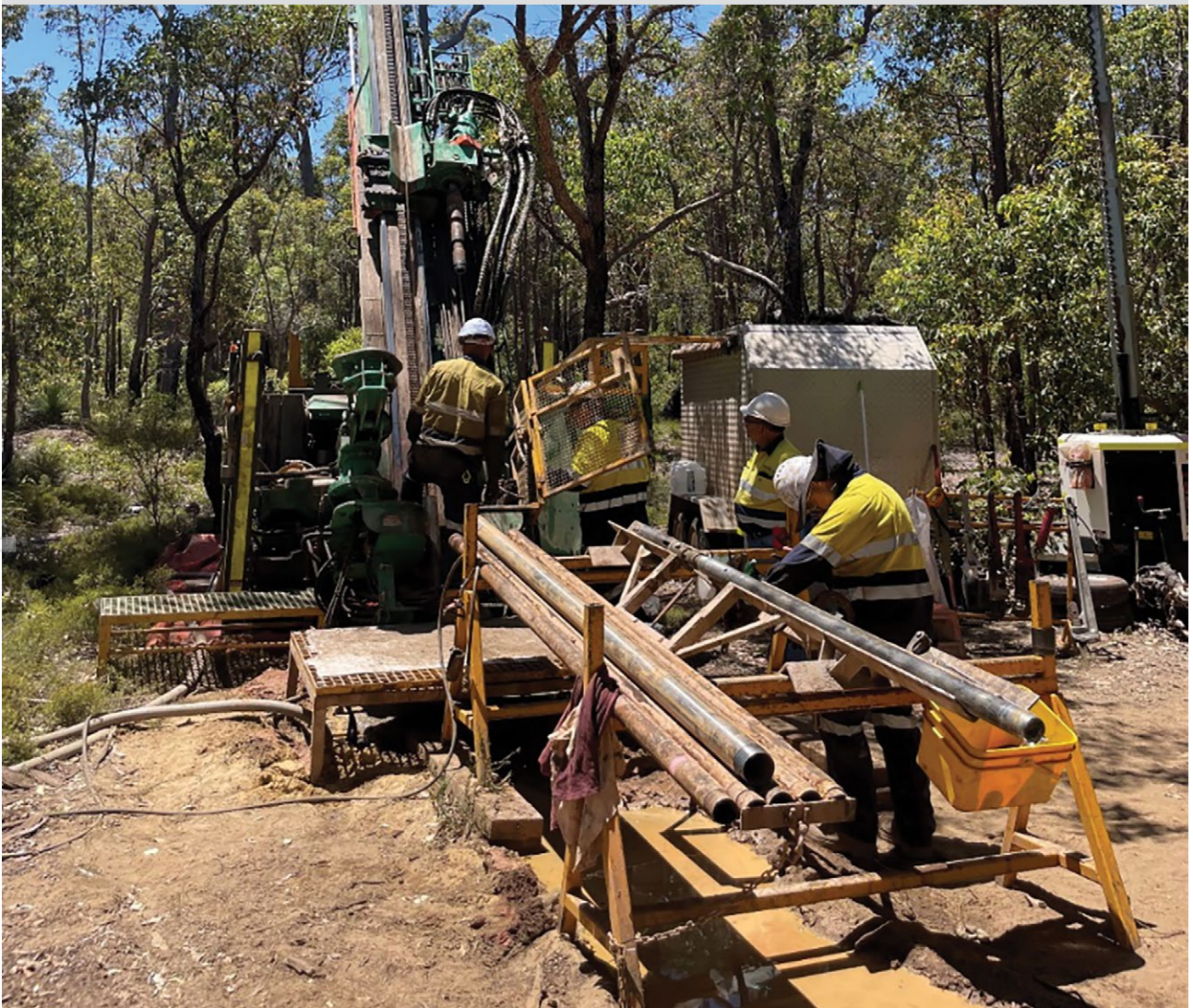
Figure 6: Diamond drilling underway at Greenbushes
