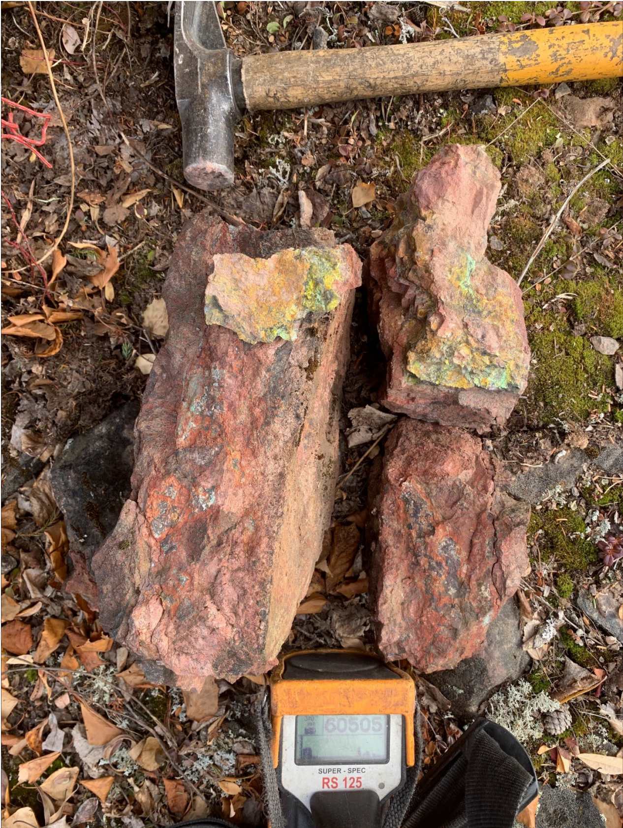
Figure 5: Uranium mineralisation in hematitic breccia from Surprise Creek Fault target
