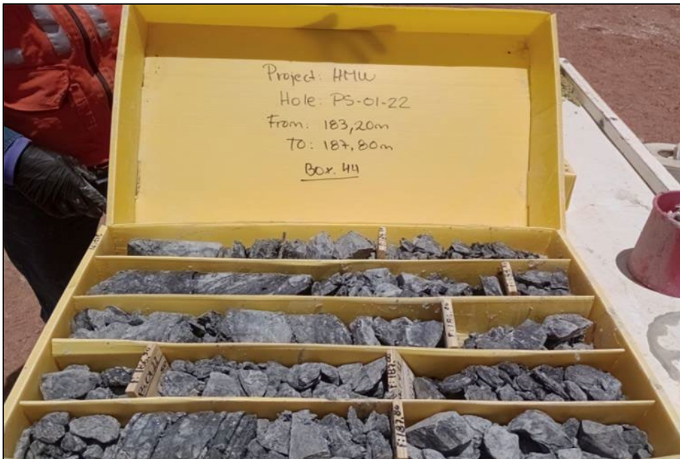
Figure 7 - Highly fractured rock core obtained from PS-01-22
