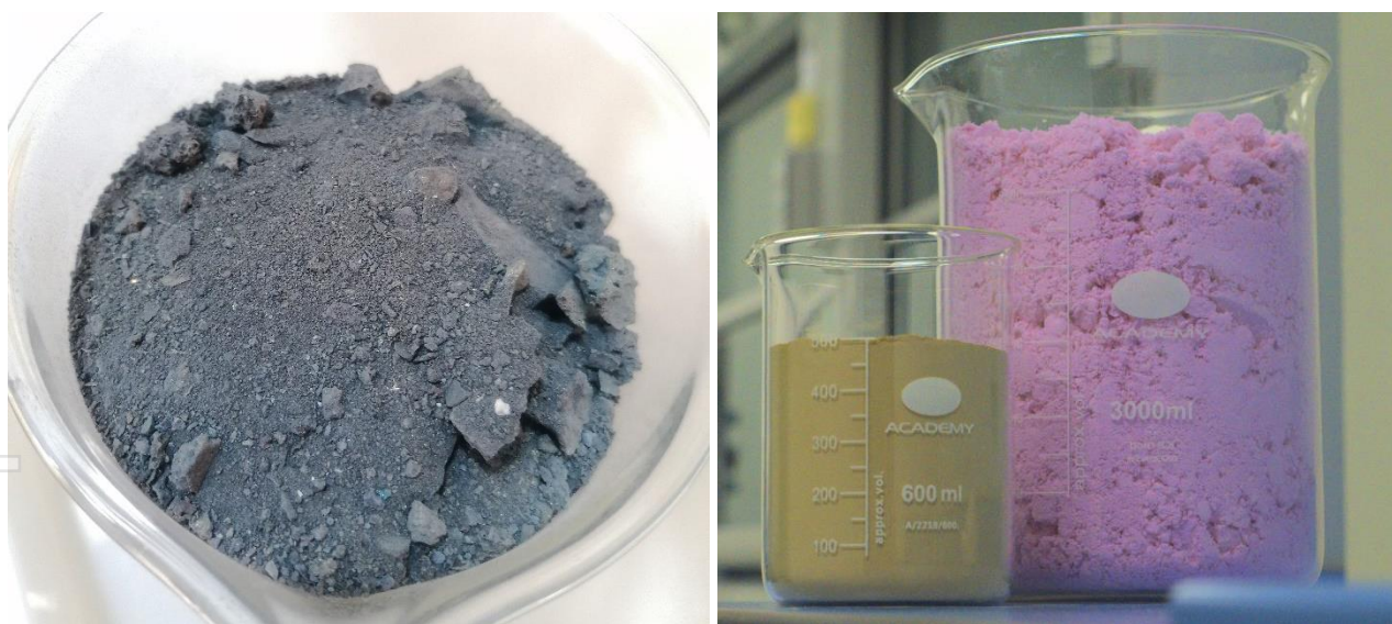
Figure 7: Swarf feedstock on the left, sourced from NdFeB metal alloy production, rich in Nd and Dy only, prior to production of intermediate products on the right – mixed Nd/Dy oxide (brown) and mixed Nd/Dy oxalate (pink).
