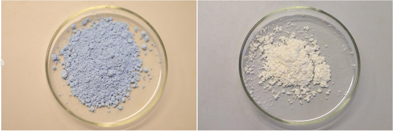
Figure 8: High purity separated oxides, showing Neodymium (Nd 2 O 3 ) (left) and Dysprosium (Dy 2 O 3 ) (right).
