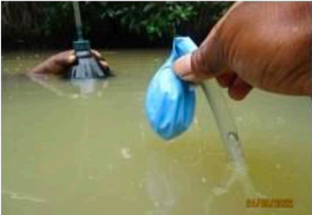
Figure 13: Collection of gas samples at Alligator Creek
