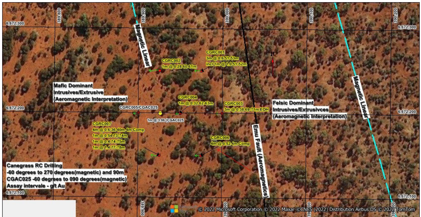
Figure 9: RC Drill Collars with significant gold intersections
