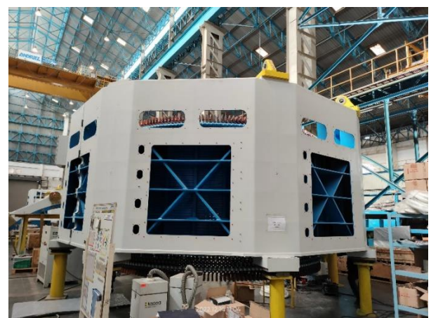
Figure 6: Andritz Hydro, Stator Frame - December 2022
