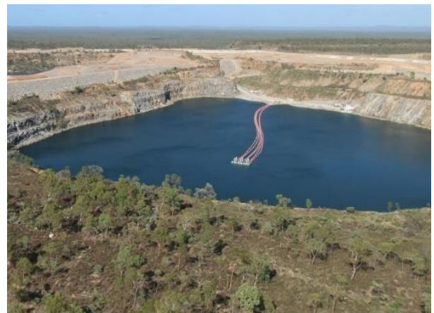
Figure 4: Dewatering pontoon and pipeline in Eldridge Pit - 21 December 2022
