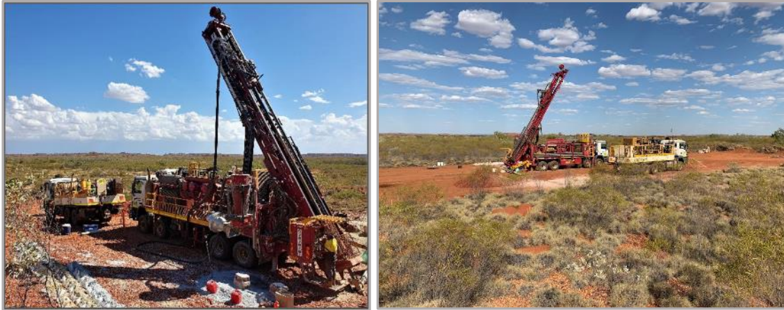
Figure 4: RC drilling rig at QXR's Turner River lithium project - Carbonate Hill area.
