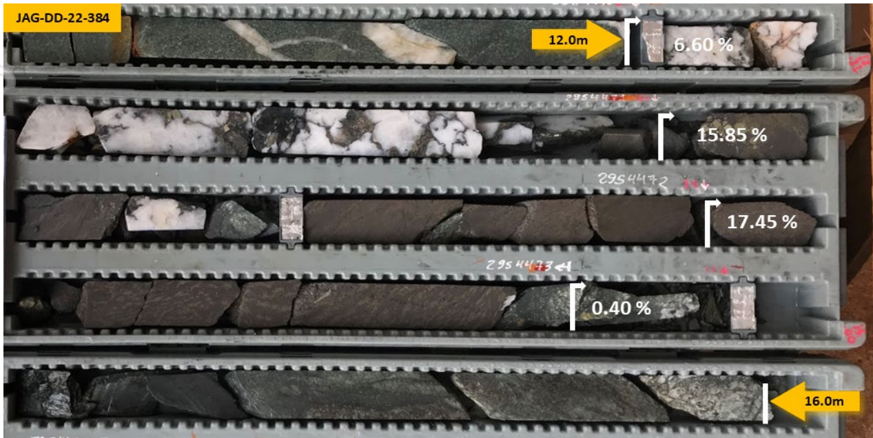
Figure 8 – JAG-DD-21-384 (Jaguar North), 12.0m to 16.0m: Semi-massive to massive sulphides (dark metallic bronze) mineralisation with magnetite alteration (black) hosted in basement gneiss. This interval returned 4.0m at 9.22% Ni, 0.19% Cu and 0.24% Co from 12.0m.
