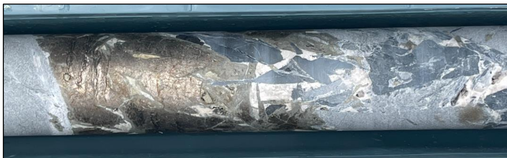
Figure 2. Photos of sulfides at 185.5m in-filling breccia fragments. Host rocks are altered metasediments. Sulfides include predominantly pyrite and sphalerite. (MPD003 - NQ diameter drill core).
