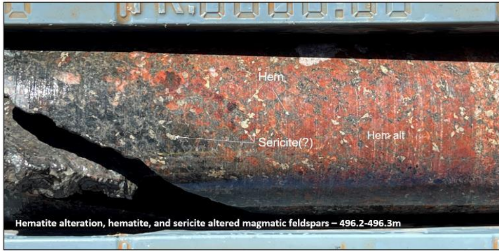
Figure 8. Hematite alteration of the igneous host rock, similar to the alteration found around other IOCG deposits in Australia
