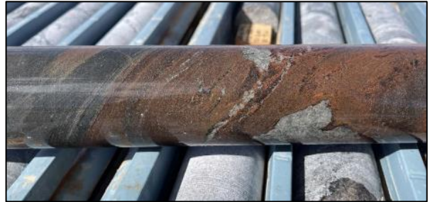
Figure 19. Photo of HQ diamond drill core CENTRAL_DD003 showing hematite staining of country rocks.
