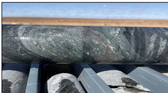
Figure 16. Initial first-pass observation of stage 2 hydrothermal alteration of host rocks. Initial observations indicate epidote-chlorite-sericite +/- actinolite and biotite alteration. Diamond HQ drill core Central_DDH003.
