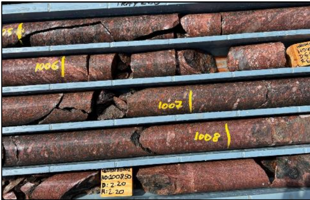
Figure 12. Felsic intrusive breccia containing significant hematite alteration with hematite and minor magnetite and pyrite within the matrix (HELIOS_DDH002). NQ size drill core. Yellow numbering represents down-hole depth in meters.
