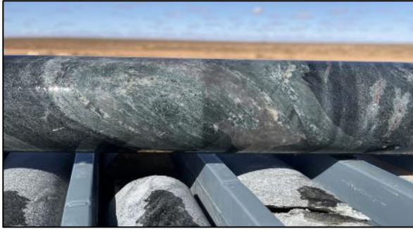
Figure 16. Initial first-pass observation of stage 2 hydrothermal alteration of host rocks. Initial observations indicate epidote-chlorite-sericite +/- actinolite and biotite alteration. Diamond HQ drill core Central_DD003.
