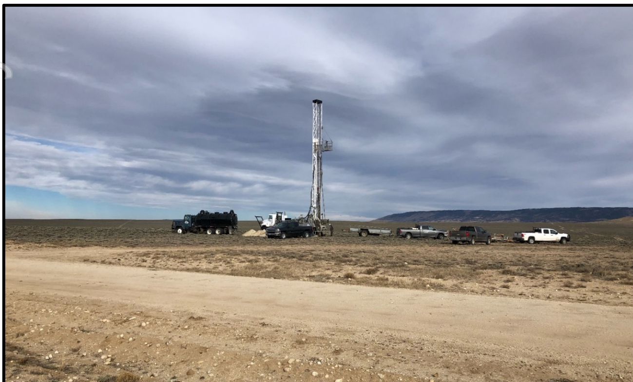
FIGURE 5: MUD ROTARY DRILL RIG OPERATING, ODIN ISR URANIUM PROSPECT, GDB WYOMING, USA
