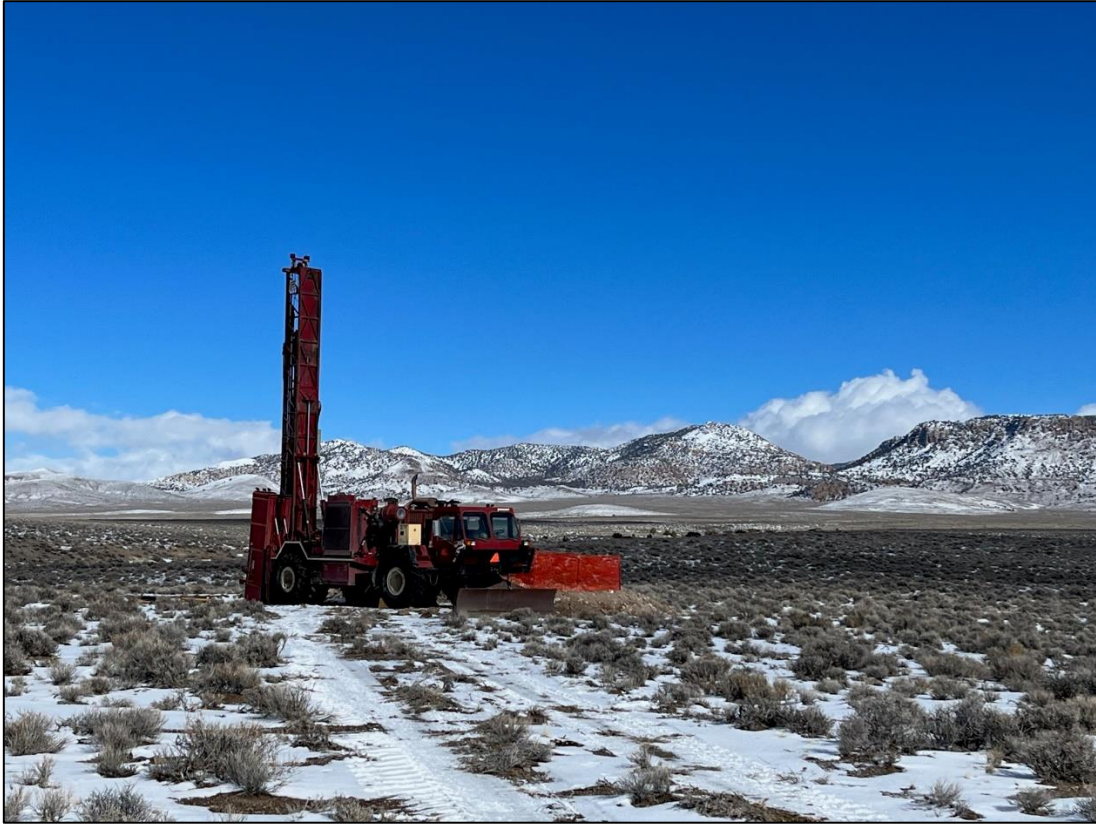
Image 1 – Reverse circulation (RC) drilling at the Nevada Lithium Project
