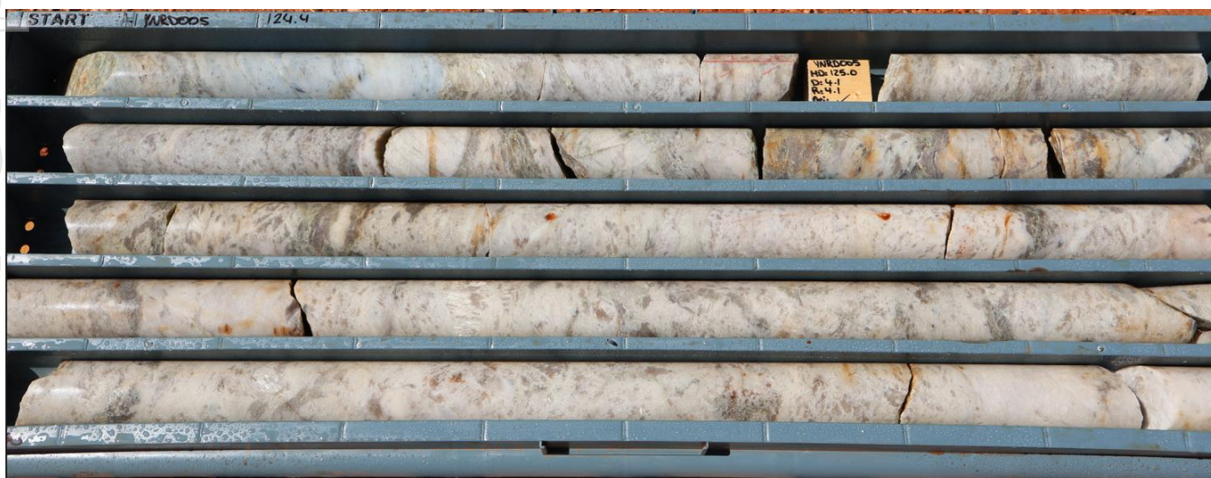
Figure 2: Photo of YNRD005 from 124.5m to 129m showing coarse grained spodumene, grade for this part of the intercept is 2.2% Li 2 O.
