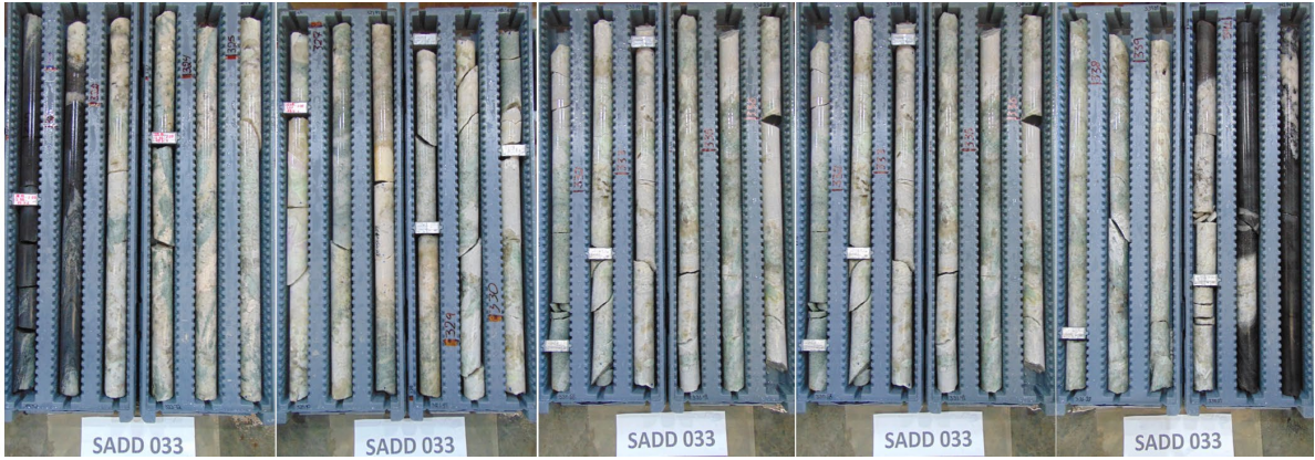
Figure 3: Colina West drill hole SADD033 – pegmatite intersection 319.40m – 341.94m (18.71m @ 1.32% Li 2 O 2 )
