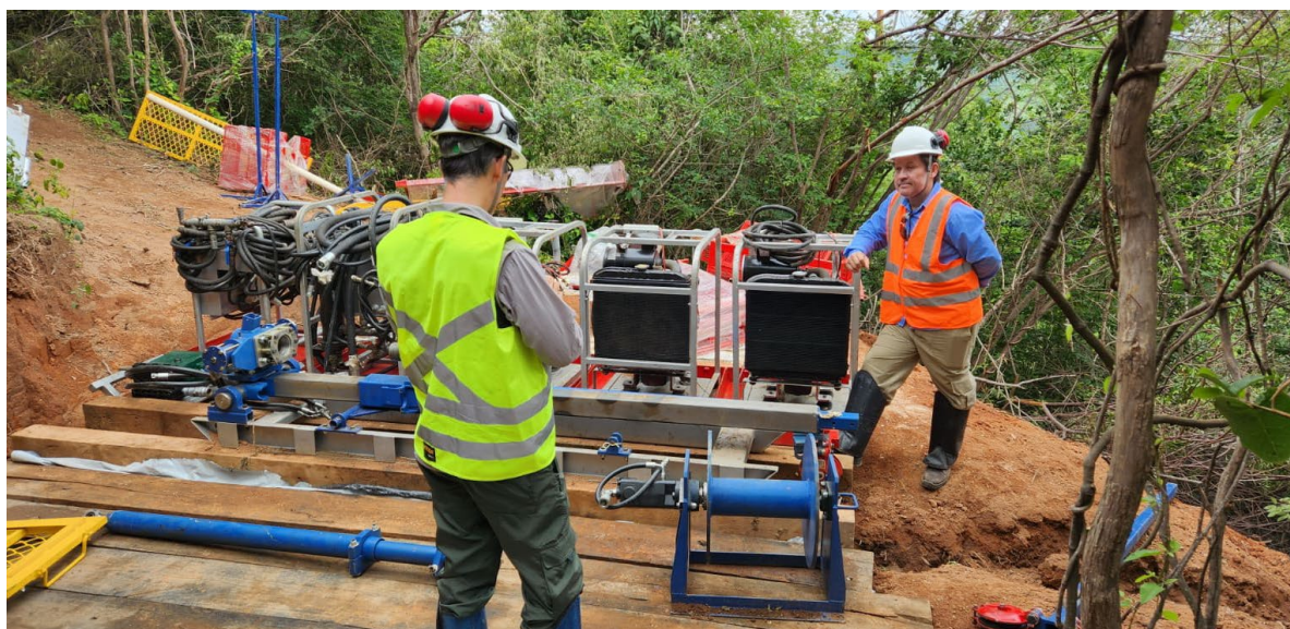
Figure 1: Man portable/ modular diamond drilling rig on site at the Colina Deposit Brazil, capable of drilling to over 400m depth, with minimal environmental impact
