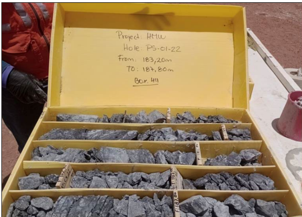
Figure 5. Highly fractured rock core obtained from PS-01-22
