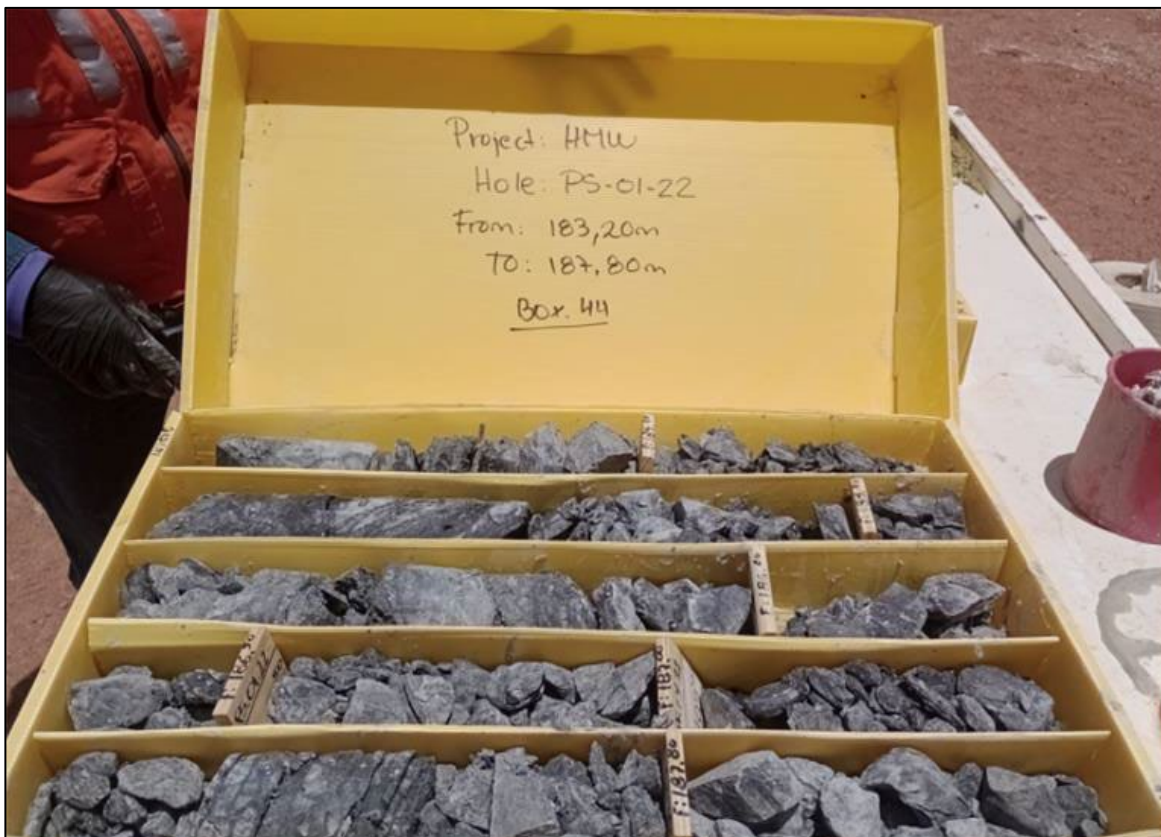
Figure 5. Highly fractured rock core obtained from PS-01-22
