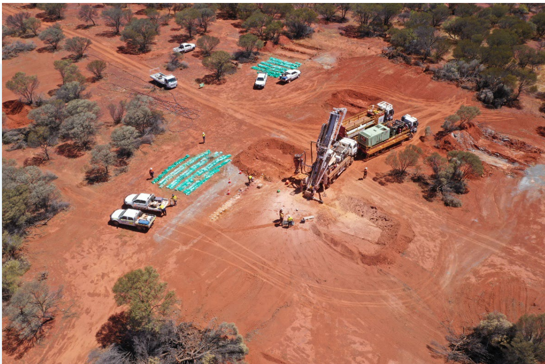
. Figure 1. Drilling underway at the Youanmi Gold Project
