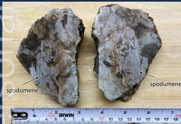
Saw cut grab sample from CV13 Pegmatite
