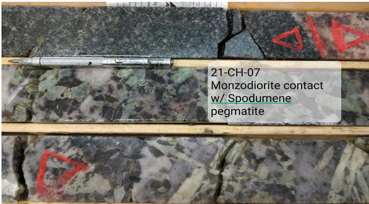
Figure 3: Close-up of 21-CH-07 Monzodiorite with fine-grained altered spodumenes (pale greenish grey crystals)
