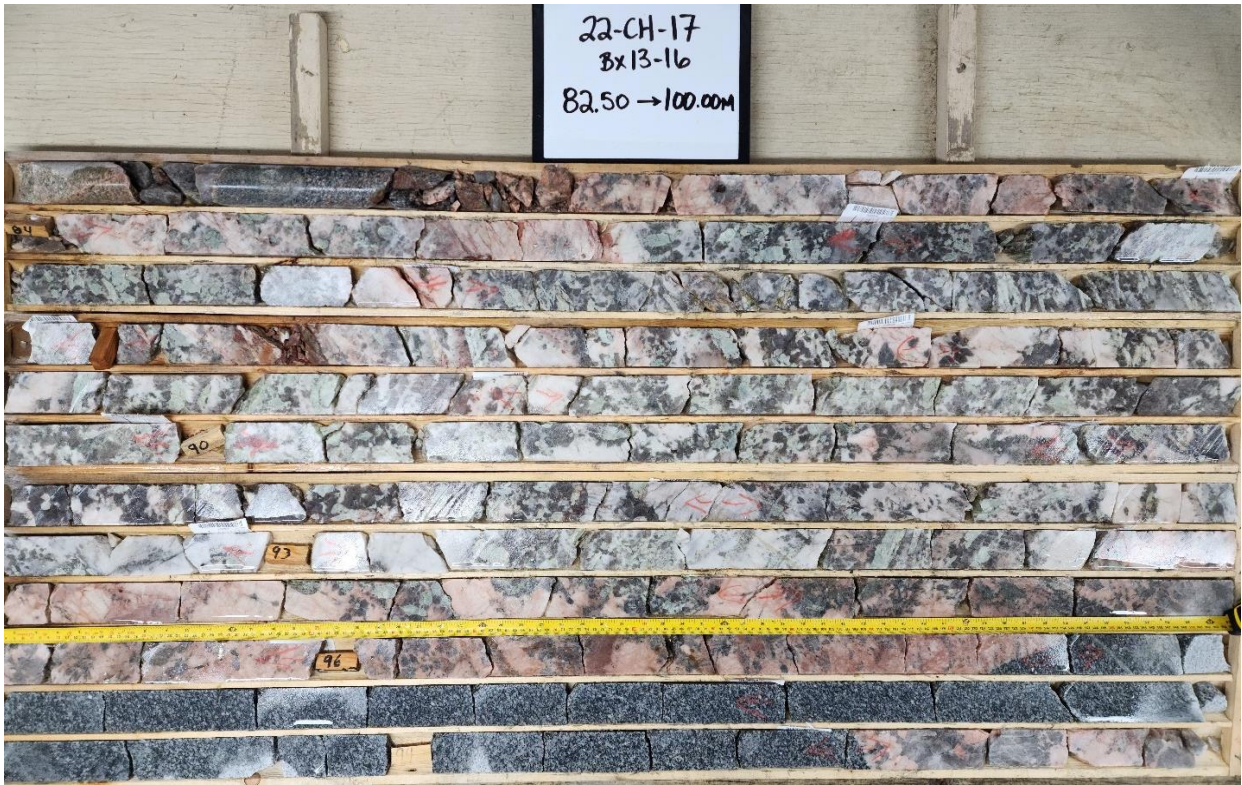
Figure 2: 22-CH-17 Interval from 82.50-100.00 m with Spodumene Pegmatite, and Granodiorite/Monzodiorite upper/lower wall rock contacts
