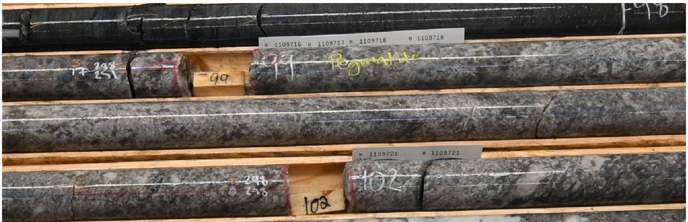
Figure 3: RL-22-041 - Whole NQ diamond core showing high density spodumene crystal laths, 15.9m @ 1.12% Li 2 O from 98.1m (incl. 6.0m @ 1.91% Li 2 O from 99.0m)
