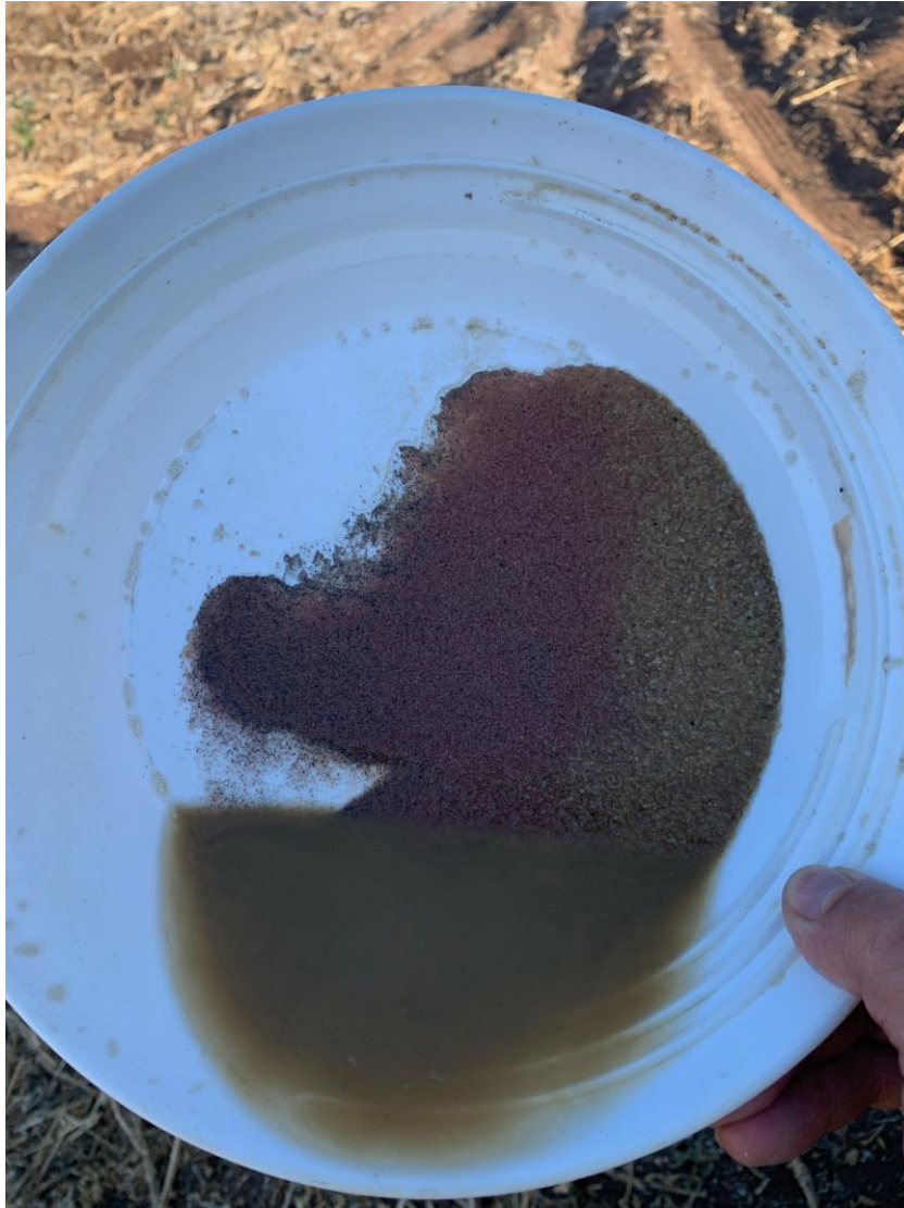
Figure 1: Visual confirmation of HM in panning of drill samples estimated at between 10 and 15% with an assemblage dominated by garnet (approximately 80 to 85%) in recently completed drilling at Port Gregory
