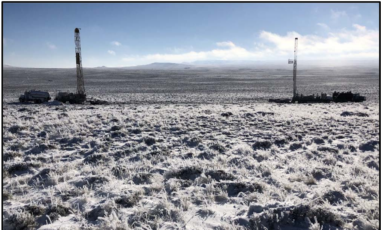
FIGURE 1. MUD ROTARY DRILL RIGS OPERATING, LOKI ISR URANIUM PROSPECT, GDB (WY).
