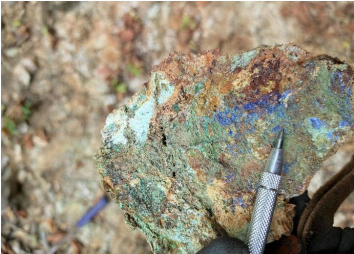
Plate 2: Hand specimen displaying azurite and malachite copper oxide mineralisation taken from the Copper Ridge prospect, Linderos Project
