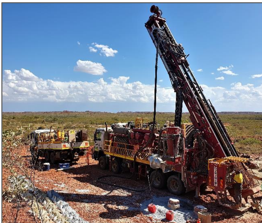
Figure 5: RC drilling rig on first hole at QXR's Turner River lithium project - Carbonate Hill area.
