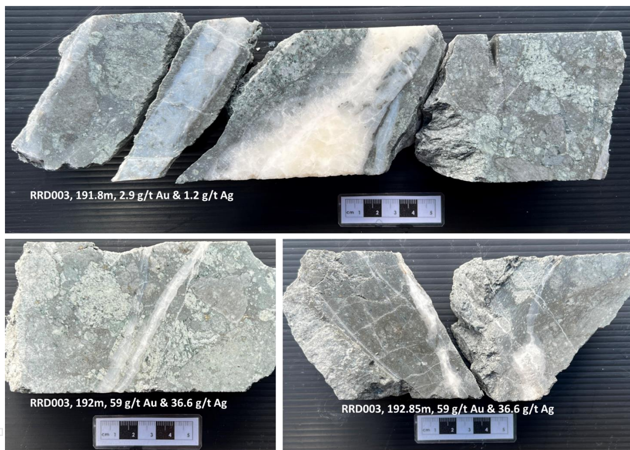
Figure 9: Core photos from deep gold intersection in RRD003. TOP: massive crystalline quartz vein with possibly later opaline blue quartz veins at margin. BOTTOM: high grade Au assay associated with the occurrence of narrow thinly banded crustiform quartz veins.
