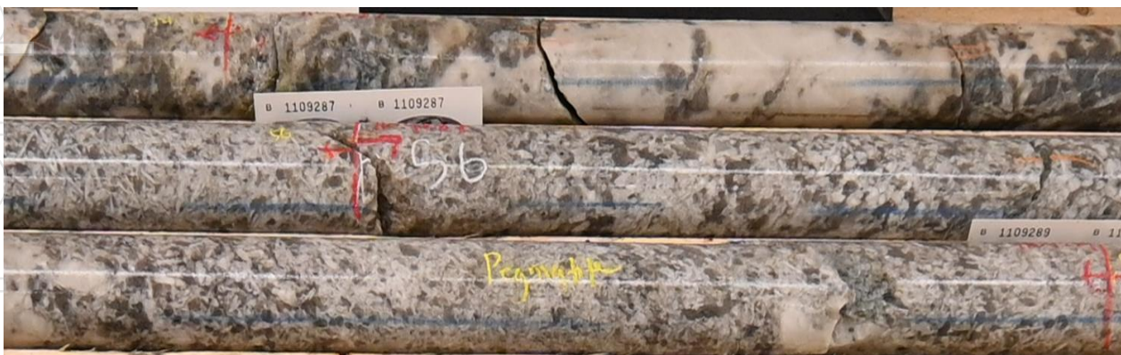
Figure 2: RL-22-017 – Whole NQ diamond core showing high density spodumene crystal laths, 6.2m @ 1.29% Li 2 O (incl. 3.5m @ 2.12% Li 2 O from 55.0m)
