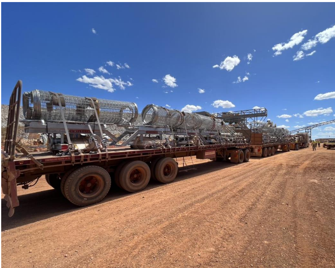
Figure 19 – Underground escapeway ladders arriving on site.
