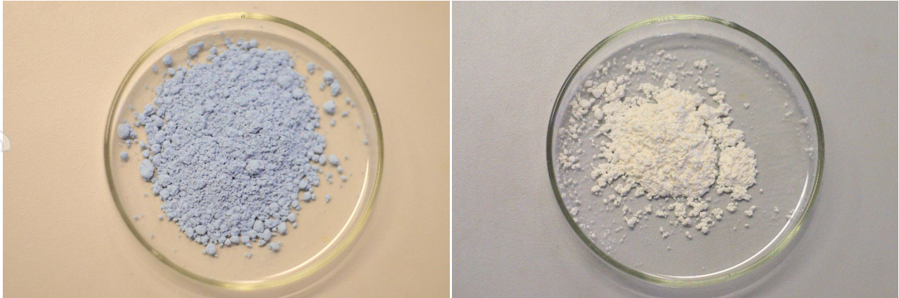
Figure 4: High purity separated oxides, showing Neodymium (Nd 2 O 3 ) (left) and Dysprosium (Dy 2 O 3 ) (right).
