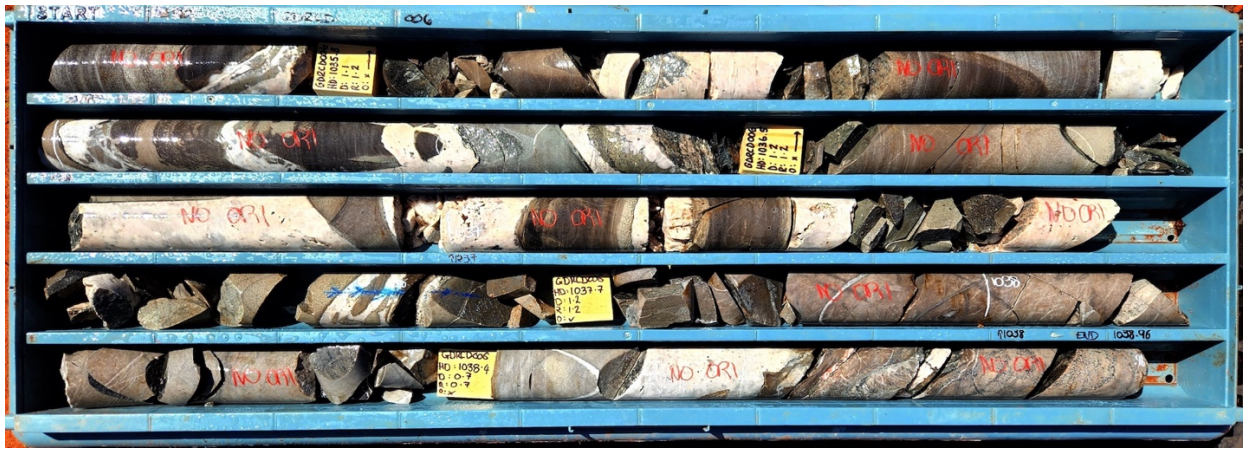
Figure 17: GRDCD006 tray at 1035.6m to 1038.9 shows vein and breccia formation with pyrite-chalcopyrite sulphide mineralisation associated with albite alteration of country rock.
