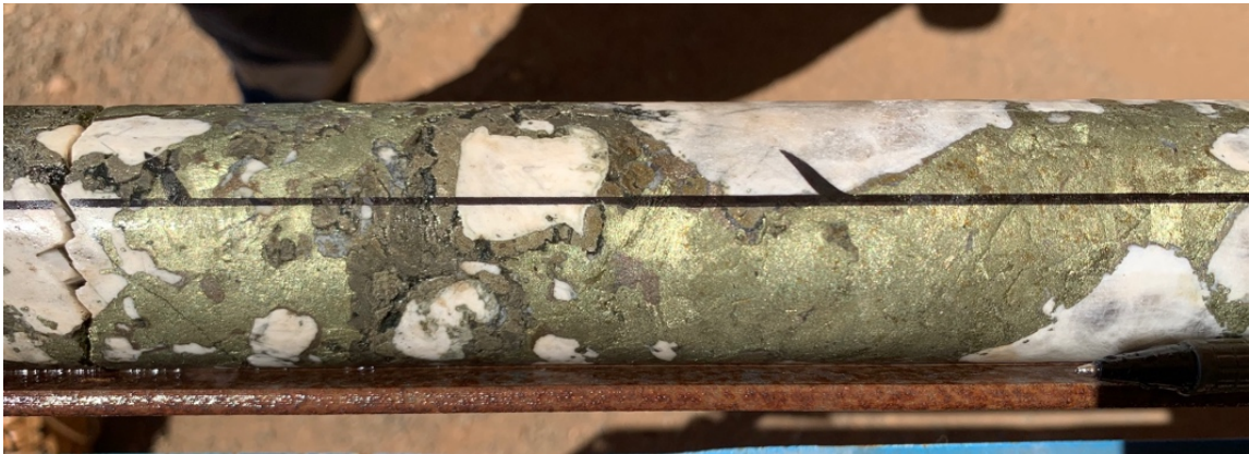
Figure 6: Hole 22PTMRD011 from 754.7 - 755.1 showing large slug of sulphide comprising of pyrite, chalcopyrite, sphalerite(?) and pyrrhotite. Copper and multi-element assays pending.
