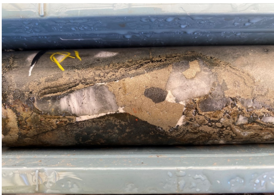
Figure 16: GRDCD006 at 960.45m close up of quartz carbonate breccia with multi-phase sulphides. Darker minerals may be tourmaline associated with the later sulphides.
