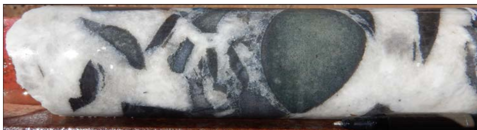
Figure 9: Hole 22PTMRD011 from 749.85 - 750.07m showing typical quartz – carbonate matrix supported jigsaw breccia that is dominant in the hole.
