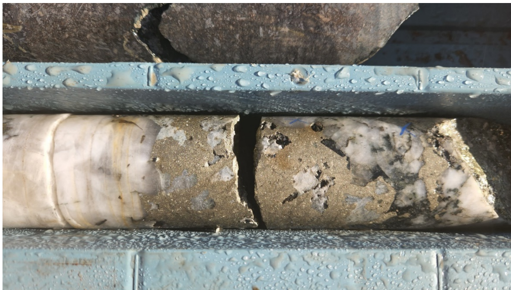
Figure 15: Hole GDRCD006 at 829.50m close up of sulphides in carbonate quartz veining. Some minor chalcopyrite is noted. Darker shades of minerals may be actinolite.
