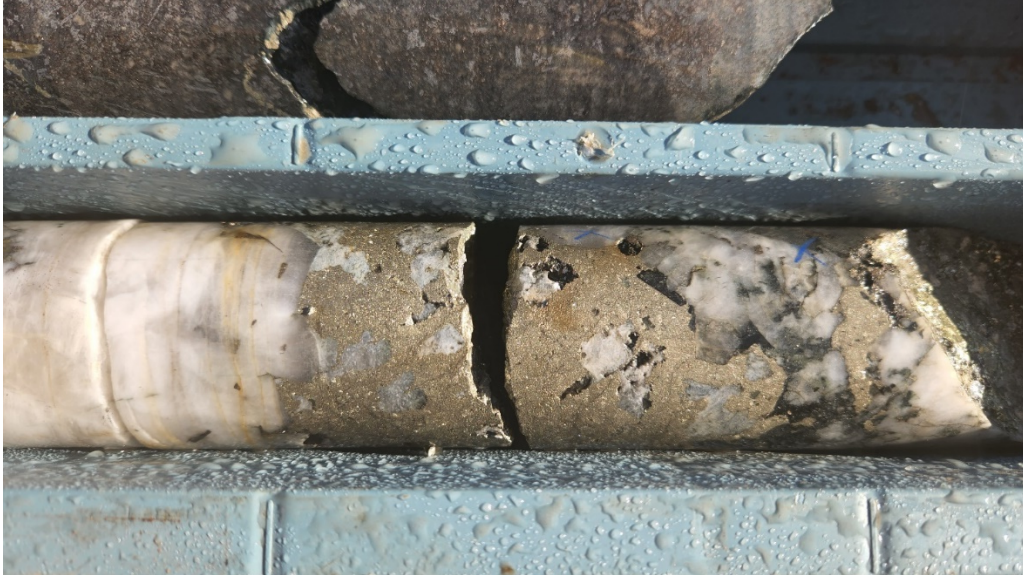
Figure 15: Hole GDRCD006 at 829.50m close up of sulphides in carbonate quartz veining. Some minor chalcopyrite is noted. Darker shades of minerals may be actinolite.
