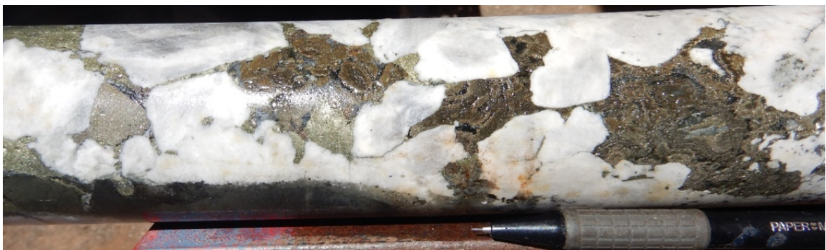
Figure 7: Hole 22PTMRD011 from 754.7 - 755.1, reverse side of Figure 6. Quartz carbonate clasts with sulphide matrix comprising chalcopyrite, pyrite, sphalerite(?) and possibly galena(?). Multi-element assays pending.
