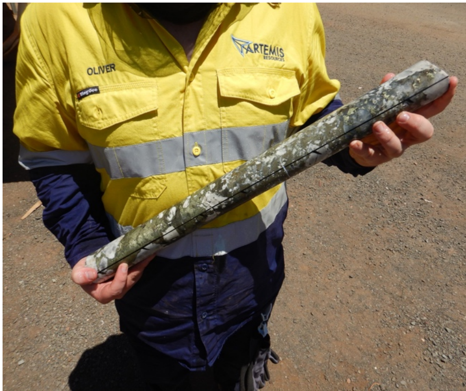
Figure 2: Core showing massive sulphide cement breccia comprising of chalcopyrite-pyrite-pyrrhotite in Hole 22PTMRD011 from 752.75 to 753.5m. Copper and multi-element assays for this core are still pending.
