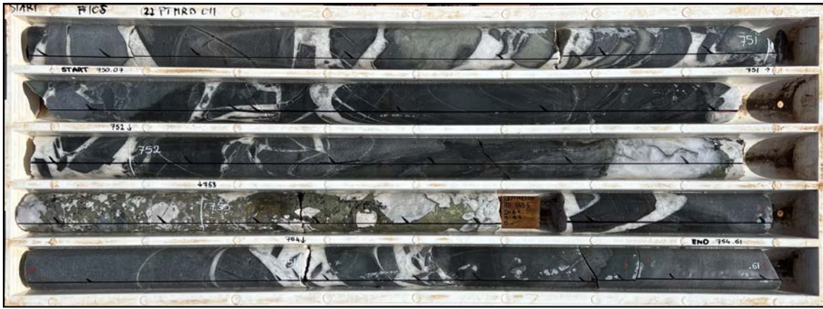
Figure 5: Hole 22PTMRD011 from 750.07m – 754.61m showing the typical quartz-carbonate breccia that dominates the hole from 705m – 826m. Drilling had intersected a section of massive sulphide within brecciated quartz and carbonate matrix from 752.7 – 753.5m. Sulphides here comprise of chalcopyrite-pyrite-pyrrhotite.
