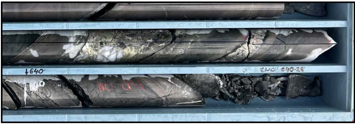
Figure 13: Hole 22PTMRD010 at 639.3 – 639.6m showing brecciated veining with chalcopyrite and pyrite mineralisation.
