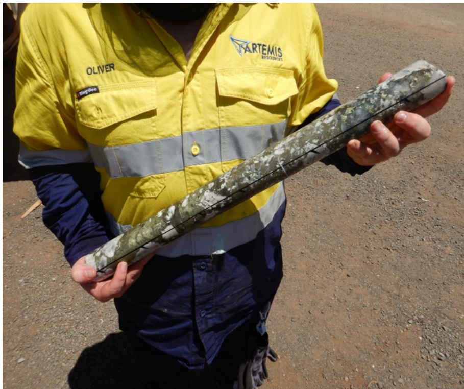
Figure 2: Core showing massive sulphide cement breccia comprising of chalcopyrite-pyrite-pyrrhotite in Hole 22PTMRD011 from 752.75 to 753.5m. Copper and multi-element assays for this core are still pending.
