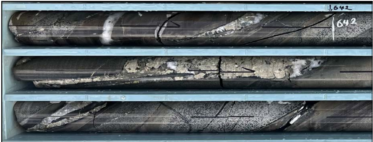
Figure 14: Hole 22PTMRD010 at 642.2 – 642.8 showing vein hosted sulphides of pyrite and chalcopyrite mineralisation. Veins of sulphide and quartz appear above and below this interval.
