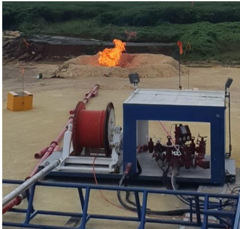
Figure 6 - Flaring operations whilst drilling Alameda-1 (Unit 3, Upper Sheet)
