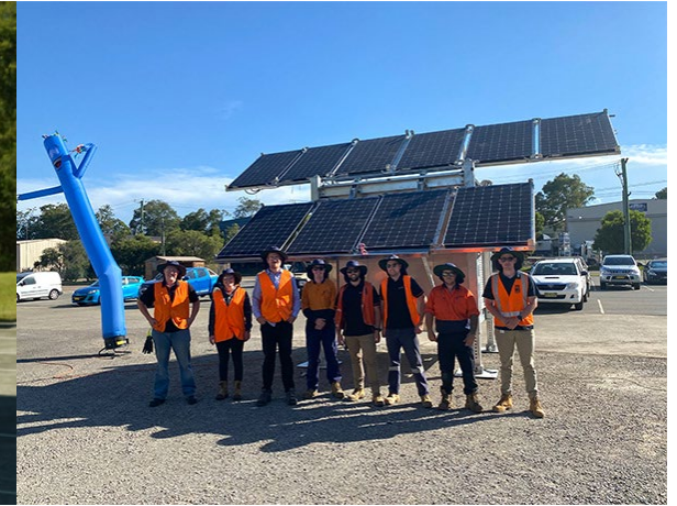
Standalone Power Systems designed to replace 'poles and wires' grid connection
