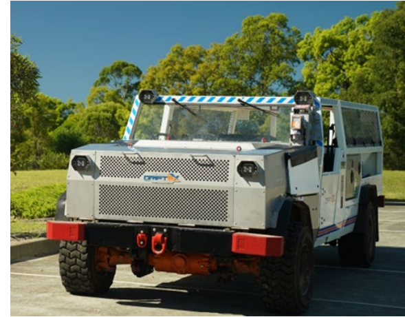
DRIFTEX is the first battery operated vehicle to operate in an intrinsically safe environment
