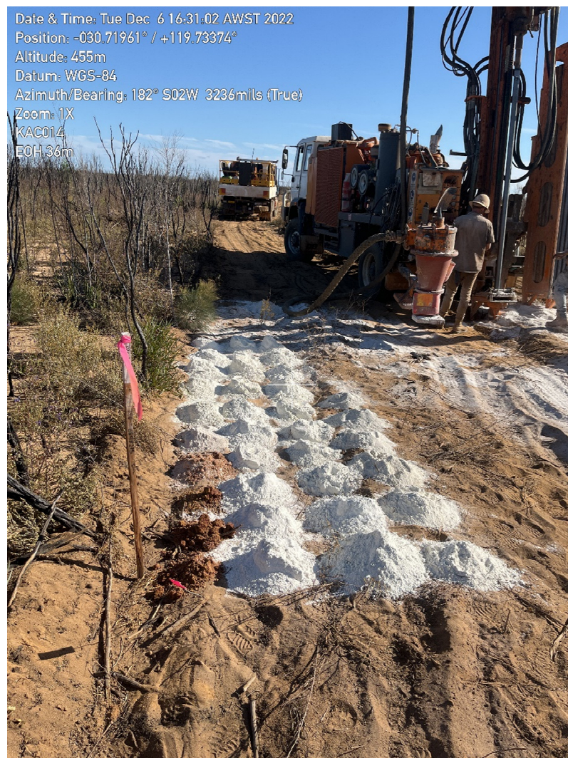
Figure 1. High quality Kaolin intersected 30m of bright white kaolin from 4m depth (KAC014).
