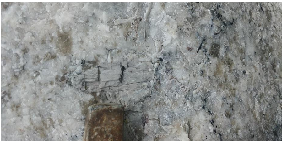
Photo 10: Spodumene crystal at the CV9 Pegmatite
