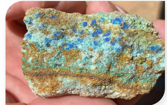
Copper oxides replacing chalcocite in outcropping sandstone.
