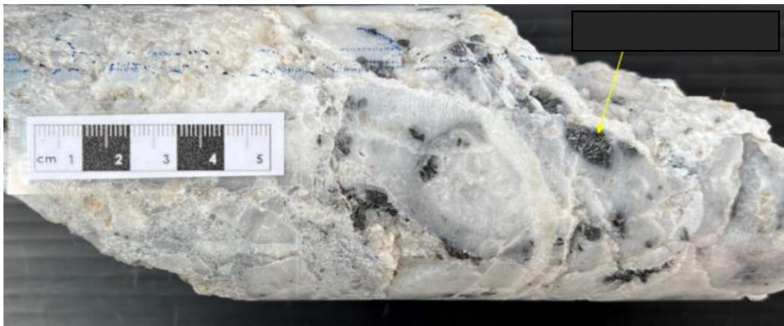
Figure 3: TOP: whole core sample of black ginguro-band in quartz vein from RDD004 104.5m. BOTTOM: whole core sample from RDD04 (109.6m) showing presence of electrum and other Ag-rich minerals indicated by yellow arrow as indicated by hard-held pXRF analyzer.
