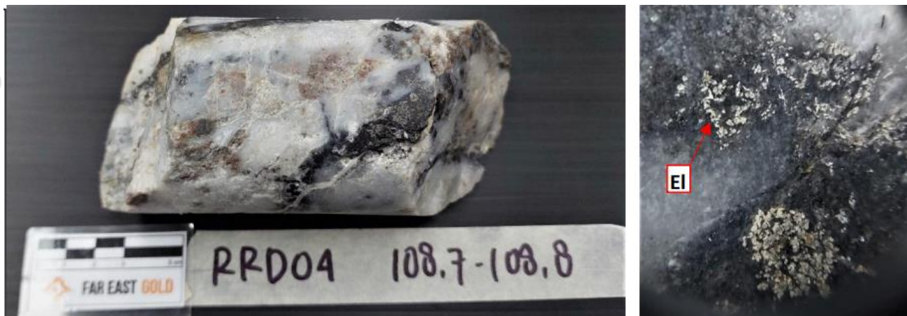
Figure 4: LEFT: Core sample from RRD004 (108.7m) quartz vein, white, colloform texture with black sulfide bends and spotted black sulfide, chalcedonic ± crystal at vugh, strong silica alteration, 3% py-cpy-sp. RIGHT: Visible gold and silver bearing minerals showing presence of electrum indicated by red arrow as indicated by hard-held pXRF analyzer.
