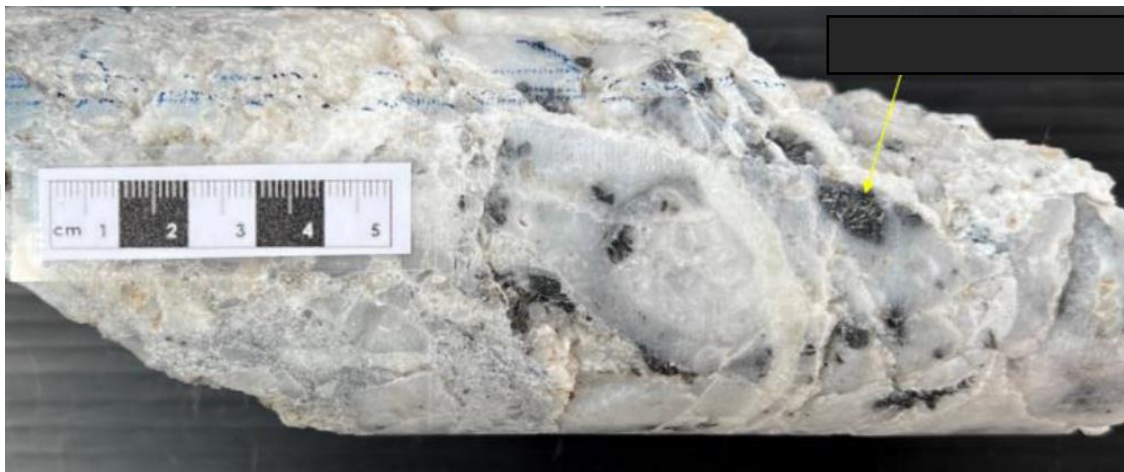
Figure 3: TOP: whole core sample of black ginguro-band in quartz vein from RDD004 104.5m. BOTTOM: whole core sample from RDD04 (109.6m) showing presence of electrum and other Ag-rich minerals indicated by yellow arrow as indicated by hard-held pXRF analyzer.
