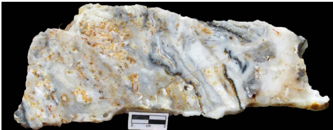
Figure 2: Sample of ginguro-banded quartz vein from artisanal mining pit in the Rek Rinti prospect. Assayed 38.14 g/t Au and 581 g/t Ag.
