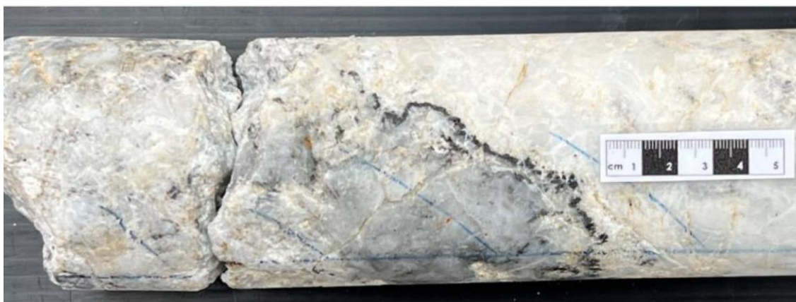
Figure 2: Sample of ginguro-banded quartz vein from artisanal mining pit in the Rek Rinti prospect. Assayed 38.14 g/t Au and 581 g/t Ag.
