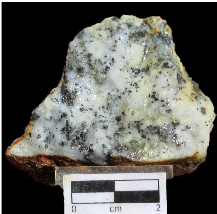
Figure 8: Photo of sulphide-rich quartz vein from southern extent of the Main Zone vein-breccia. Sample assayed; 119 g/t Au, 361 g/t Ag, 3.39 % Cu, 3.9 % Pb and 5.16 % Zn
