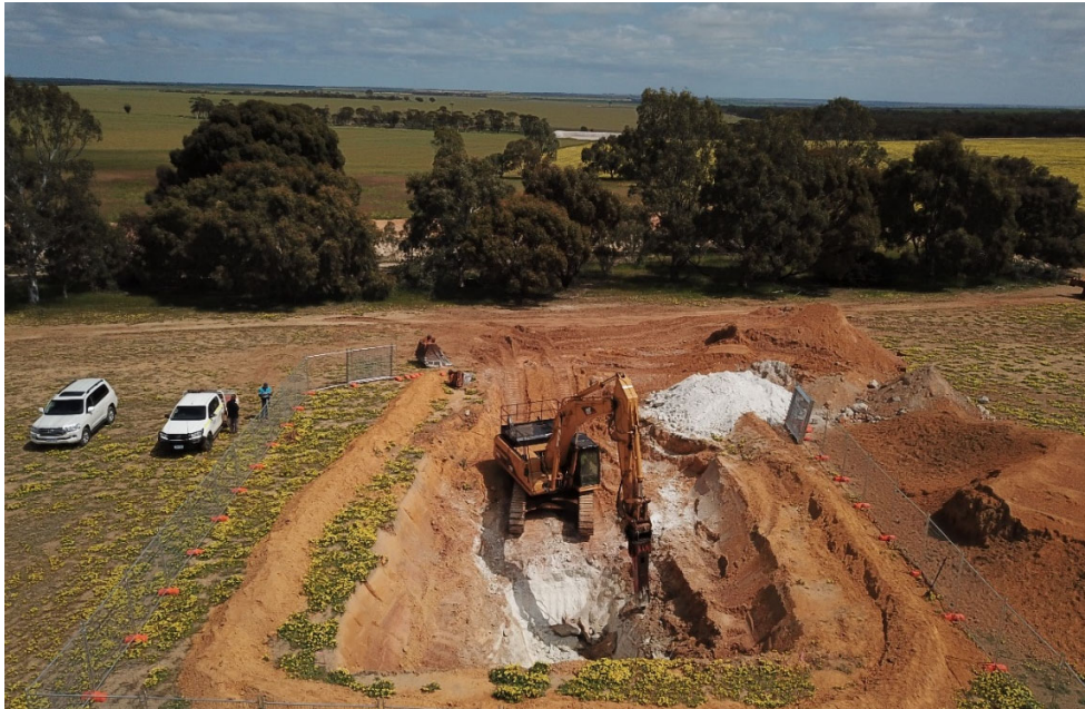
Figure 2: Bulk sample test pit showing thin colluvial cover and white kaolinitic saprolite clays
