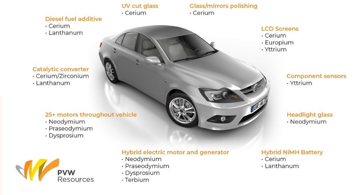
Figure 6: Rare earth elements used in electric vehicles
