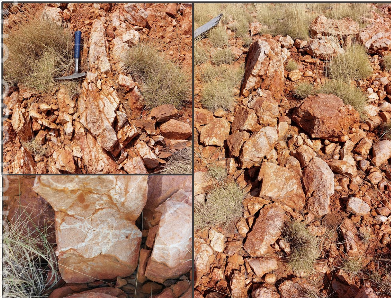
Figure 2: Quartz breccia outcrop, the surface expression of a structure that is interpreted to extend beneath Watts Rise REE mineralisation.
