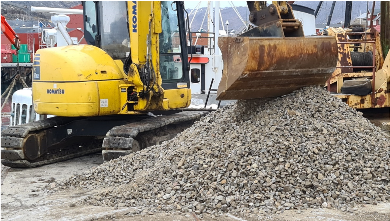
Figure 5: Crushing material from the Ivigtût waste dumps in Greenland down to 30mm.
