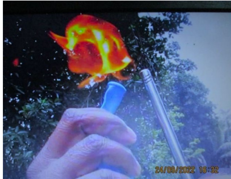
Field-test of gas bubbling from reservoir
