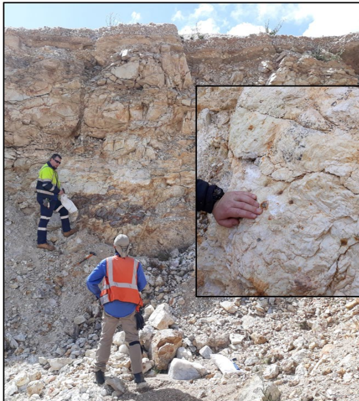
Figure 5. Quarry wall showing albite pegmatite spotted with xenotime with distinctive rusty (preferentially weathered) haloes.
